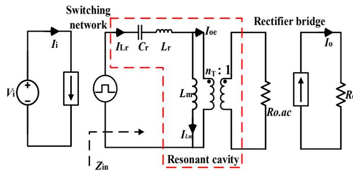
Figure 8. Steady-state equivalent circuit of SDBuck-LLC.
