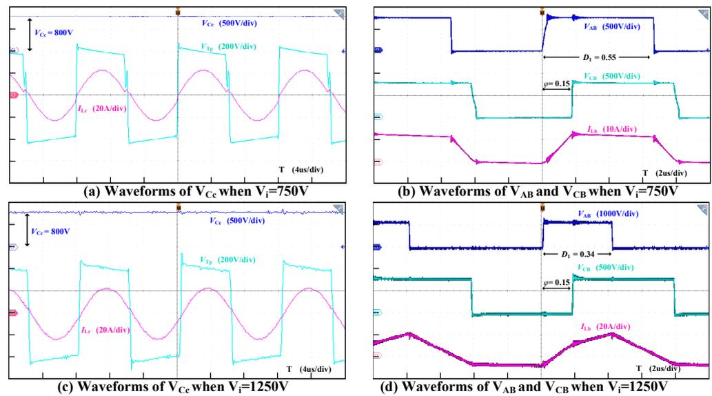
Figure 14. Steady-state experimental waveform of SDBuck-LLC with an output power of 6.25 kW under different  $V_i$ .
