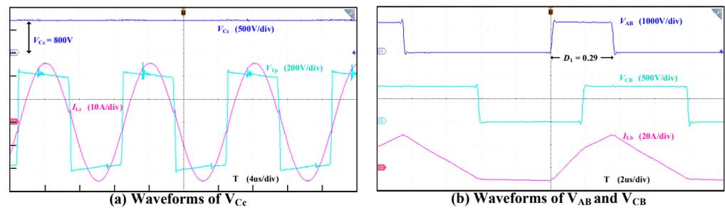
Figure 15. Steady-state experimental waveforms of SDBuck-LLC with an output power of 6.25 kW and input voltage of 1400 V.
