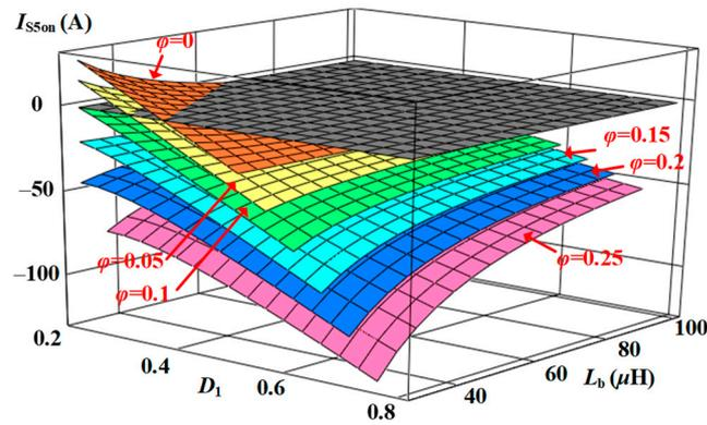
Figure 10. The relationship between  $I_{S5on}$  and  $D_1, L_b$  under different phase shifts  $\varphi T_s$ .
