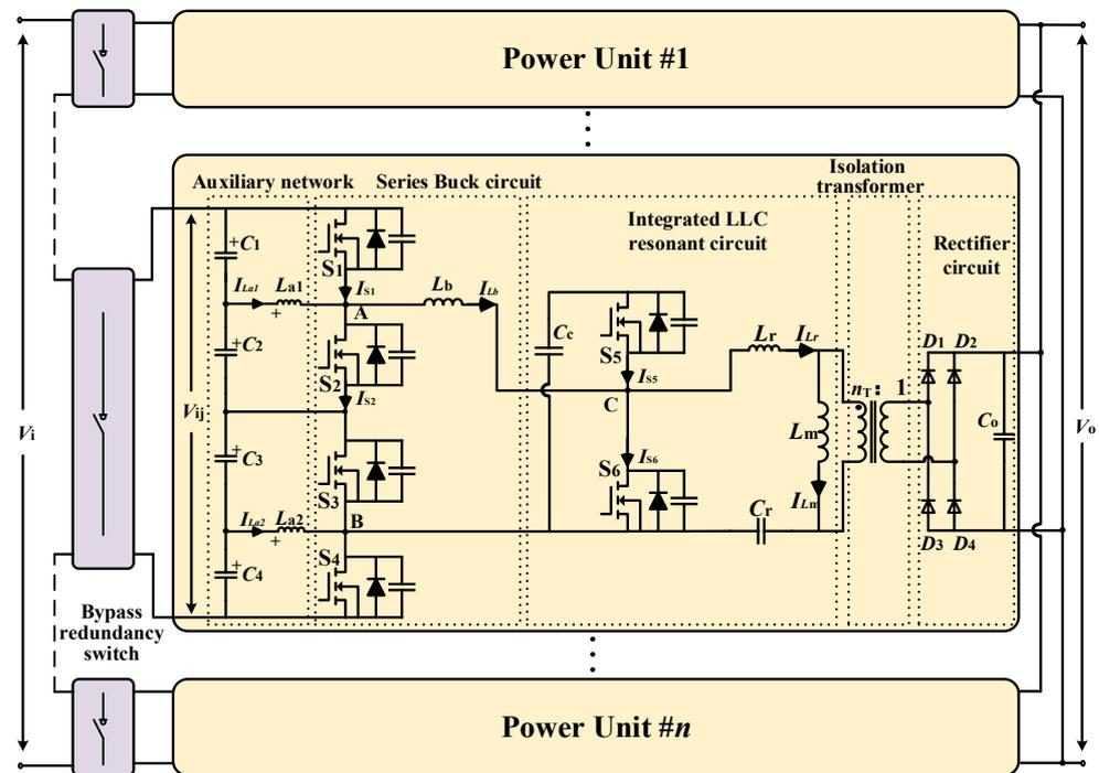
**Figure 1.** Modular combined DC-DC converter based on Buck-LLC integration.
