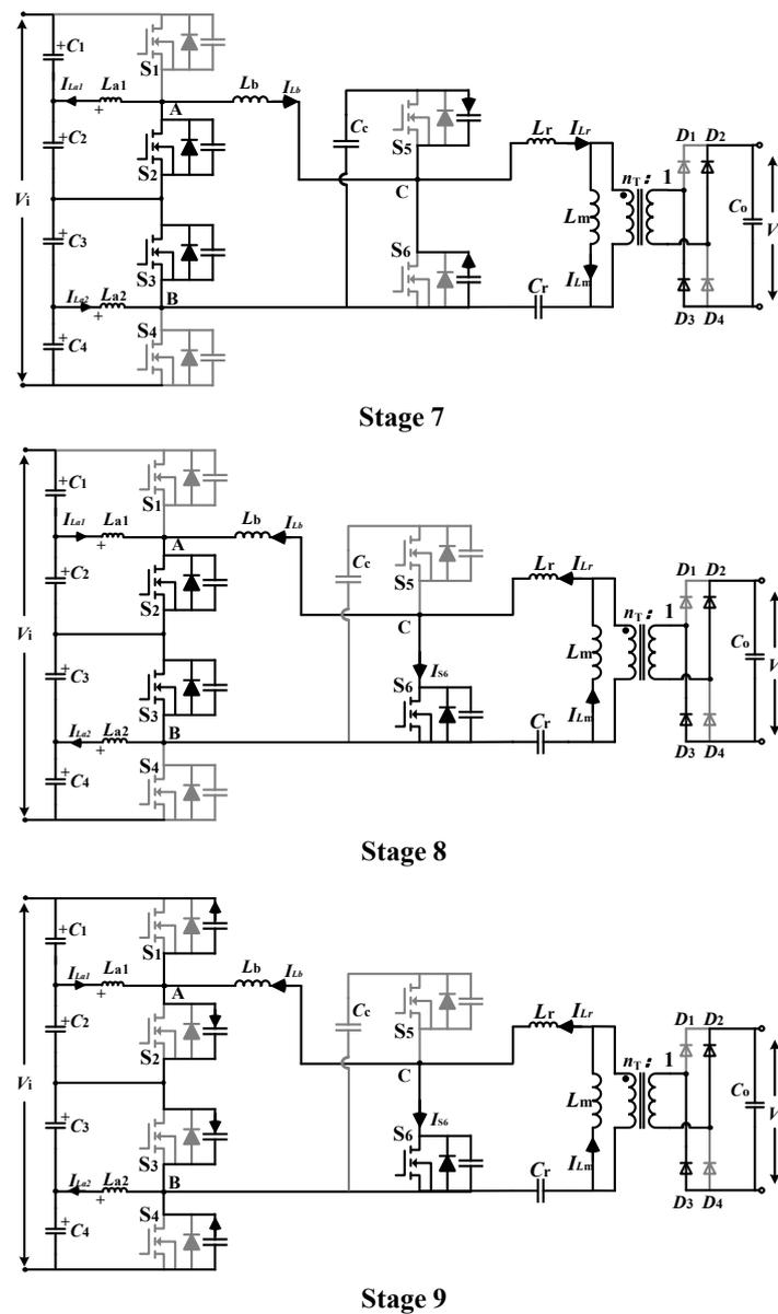
Figure 7. Equivalent circuits of stage 7, stage 8, and stage 9 in mode X1.
