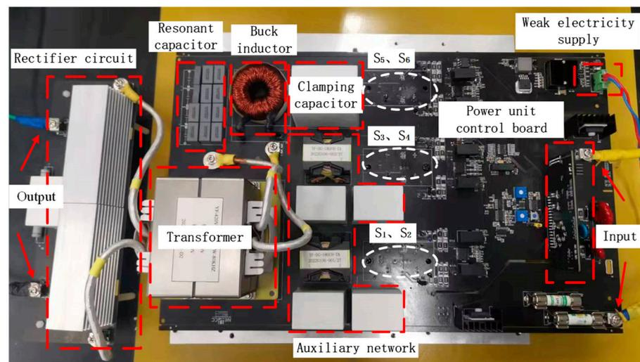
**Figure 13.** Experimental prototype of SDBuck-LLC.
