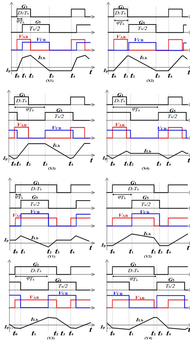
Figure 2. Waveforms of each operational mode of SDBuck-LLC.
