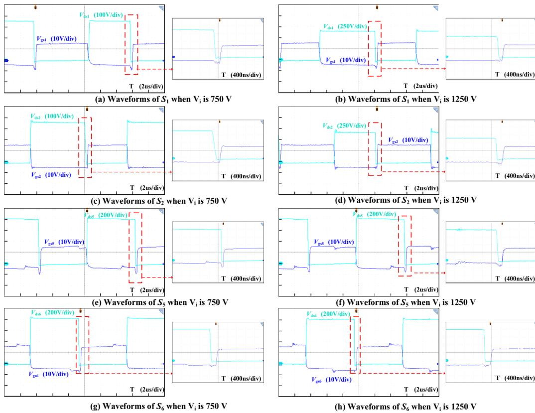
Figure 17. ZVS waveforms of each switch under light load and different input voltages  $V_i$ .
