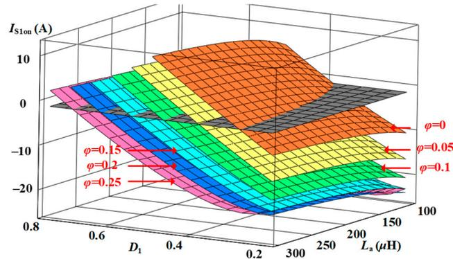
Figure 12. The relationship between  $I_{S1on}$ ,  $I_{S4on}$ , and  $D_1$ ,  $L_b$  under different phase shifts  $\varphi T_s$ .
