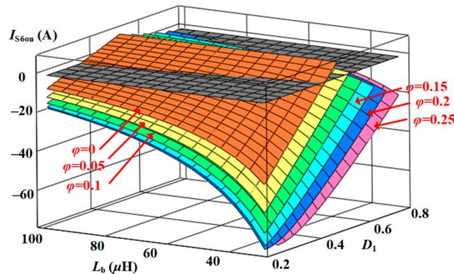
Figure 11. The relationship between  $I_{S6on}$  and  $D_1, L_b$  under different phase shifts  $\varphi T_s$ .
