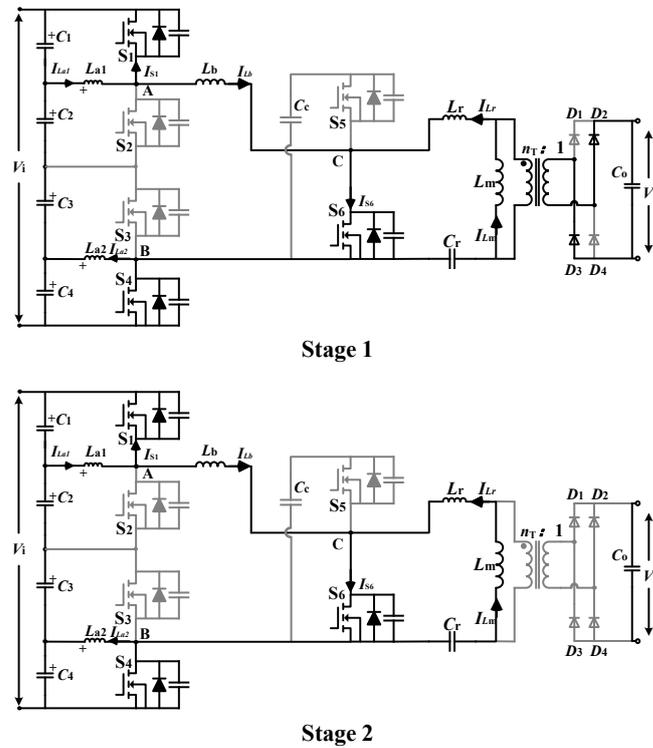
Figure 4. Equivalent circuits of stage 1 and stage 2 in mode X1.
