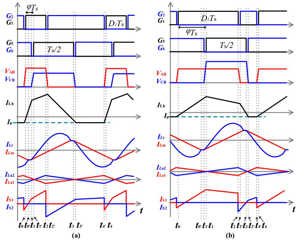
Figure 3. Key voltage and current waveforms of SDBuck-LLC (a) mode X1 and (b) mode Y2.
