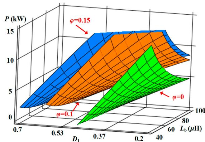
**Figure 9.** The relationship between power  $P$  and  $D1$ ,  $L_b$  under different phase shifts  $\varphi T_s$ .
