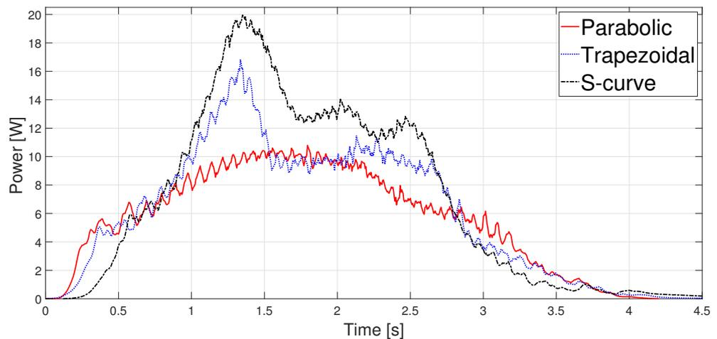
Figure 25. Power estimated with a load of 9 kg.
