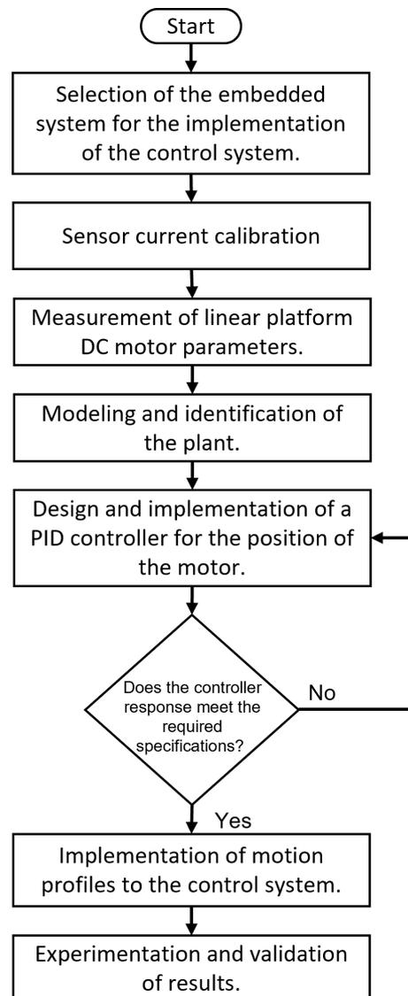
**Figure 4.** Design stages of a motion controller.
