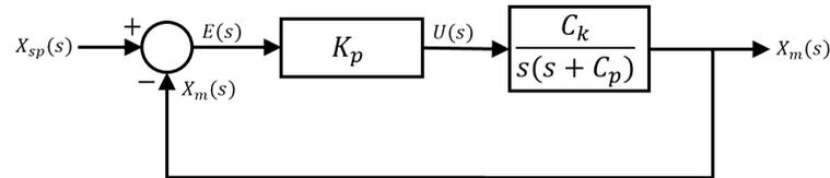
Figure 5. Block diagram of the system used for identification.
