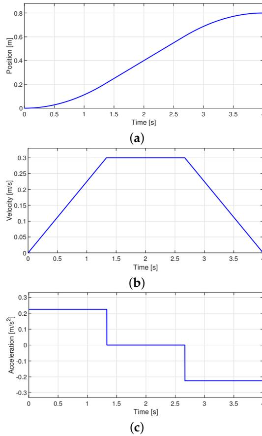
**Figure 2.** Trapezoidal velocity profile: (a) Position, (b) Velocity, and (c) Acceleration.
