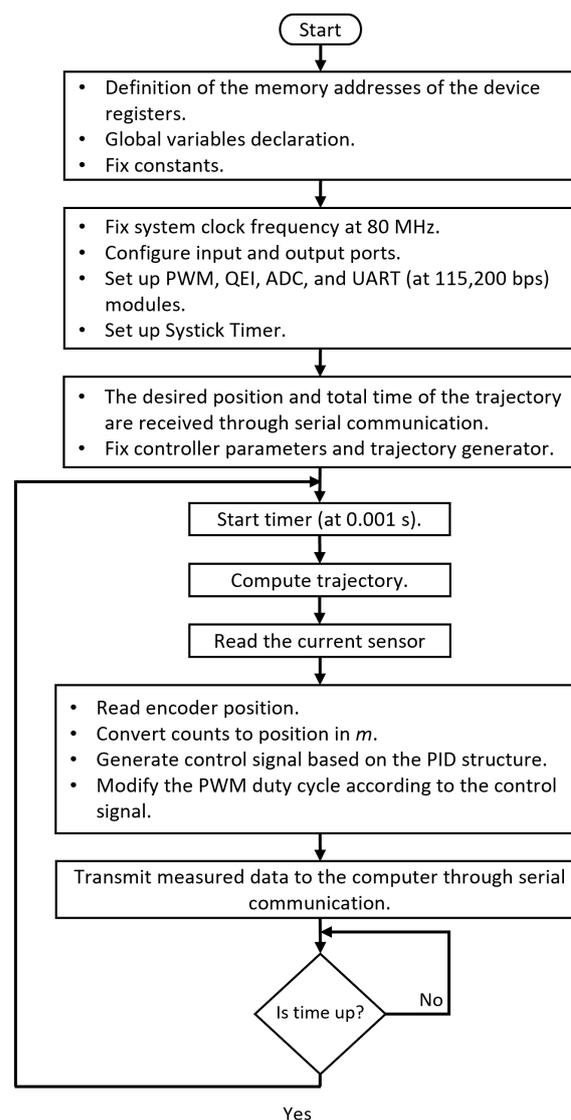
Figure 9. Flowchart of the algorithm used for the microcontroller programming.
