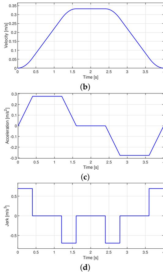
**Figure 3.** S-curve velocity profile: (a) Position, (b) Velocity, (c) Acceleration, and (d) Jerk.
