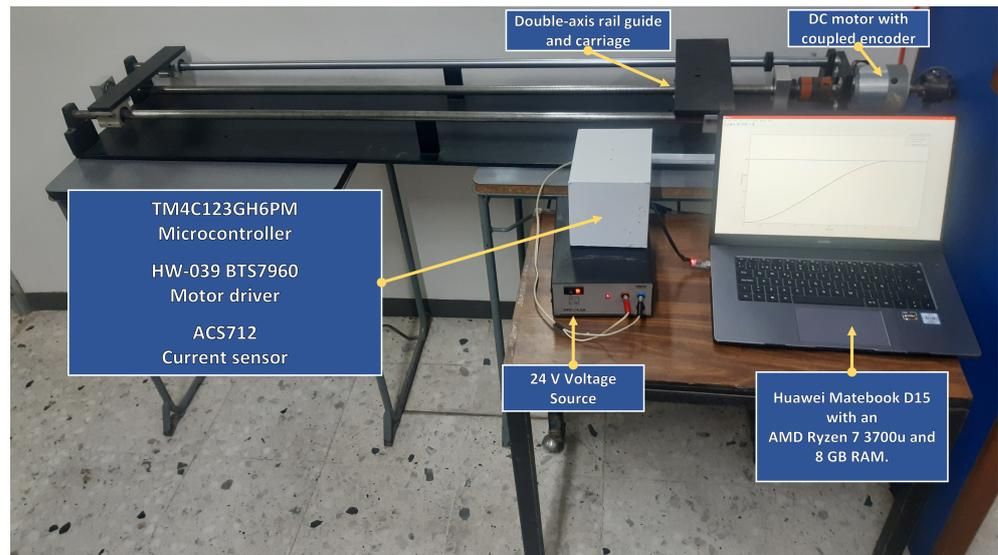
Figure 13. Linear plant used for the experimentation.
