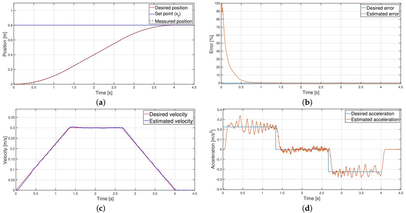
**Figure 17.** Trapezoidal velocity profile: (a) Position, (b) Error (c) Velocity, and (d) Acceleration.
