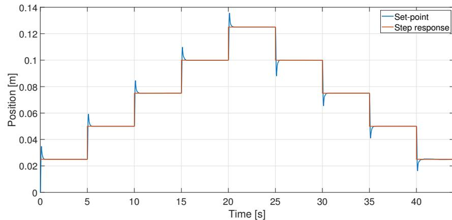
Figure 14. Test of steps response to prove the robustness of the controller.
