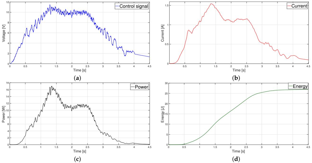
Figure 20. S-curve velocity profile: (a) Control signal, (b) Current (c) Power, and (d) Energy.
