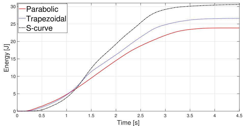
Figure 26. Energy estimated with a load of 9 kg.
