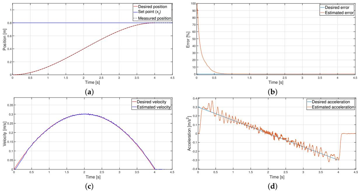
Figure 15. Parabolic velocity profile: (a) Position, (b) Error (c) Velocity, and (d) Acceleration.
