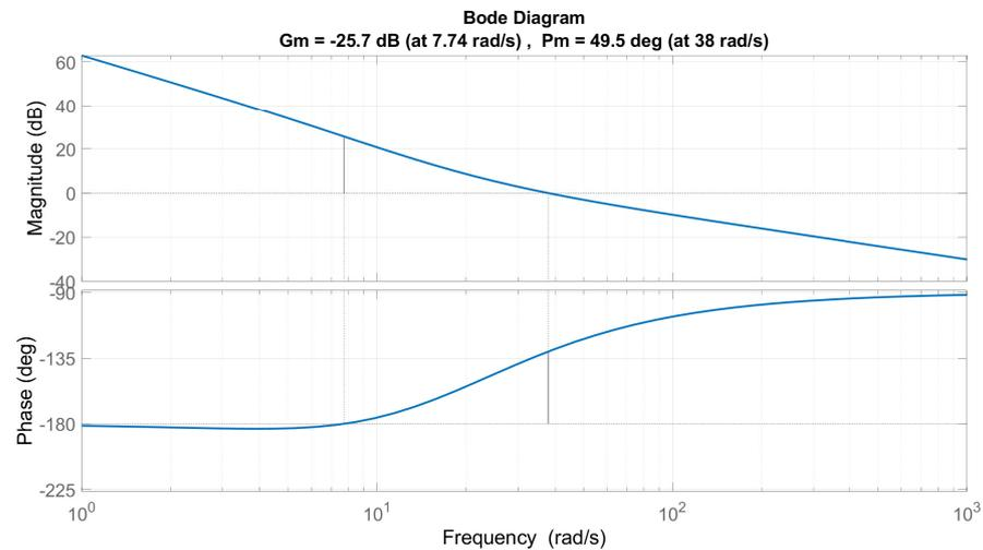
Figure 11. Bode diagram of the control system.
