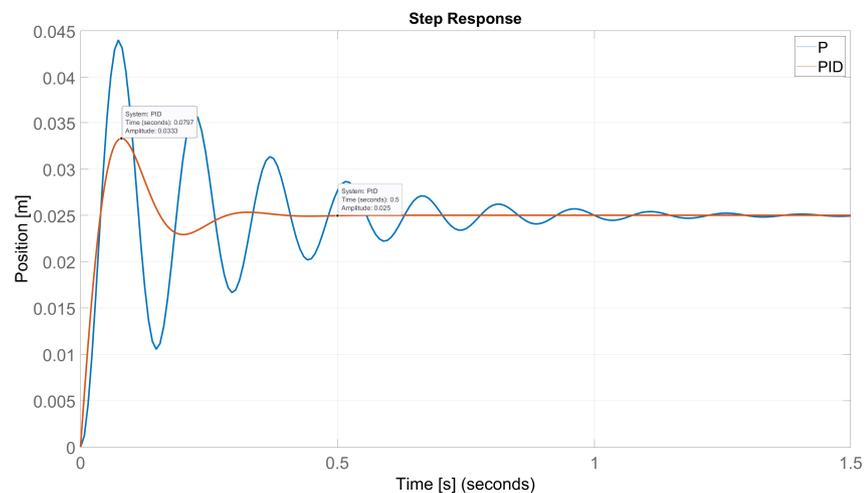
Figure 12. Time response of the system to a step input, applying a PID controller.
