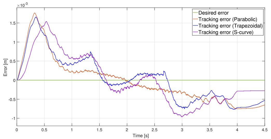
Figure 21. Real error position with a load of the three position profiles.
