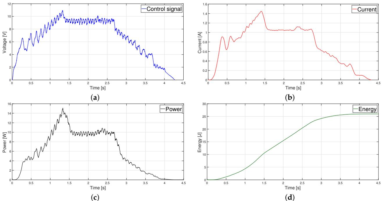
**Figure 18.** Trapezoidal velocity profile: (a) Control signal, (b) Current (c) Power, and (d) Energy.
