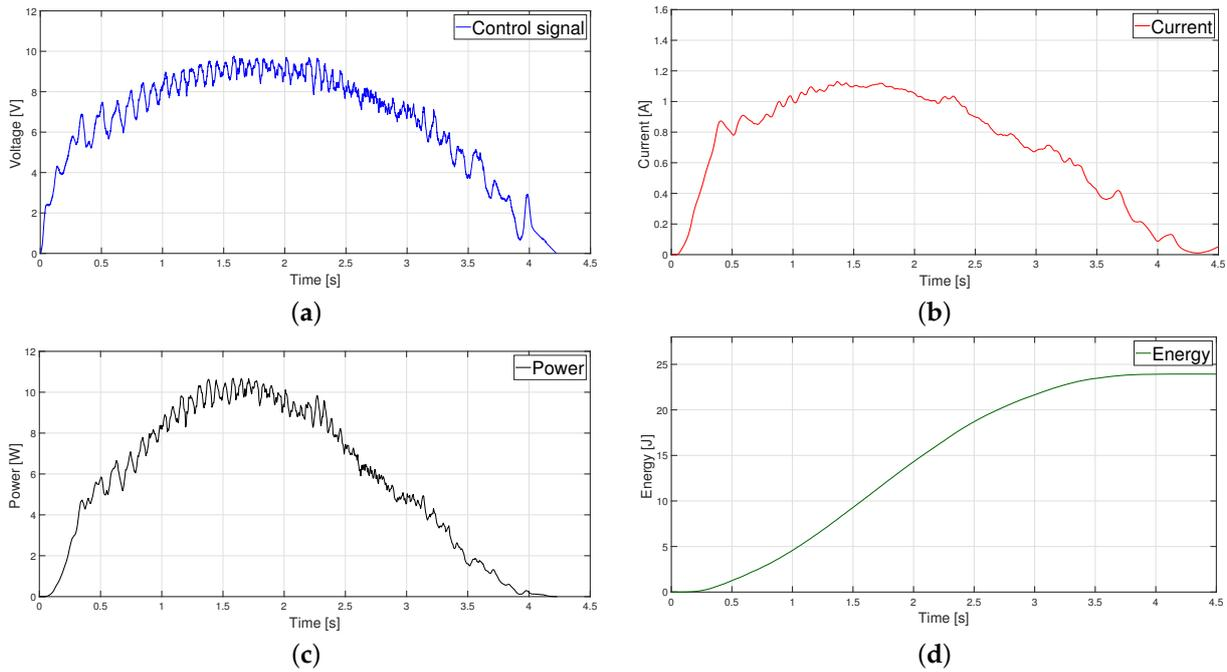
**Figure 16.** Parabolic velocity profile: (a) Control signal, (b) Current (c) Power, and (d) Energy.
