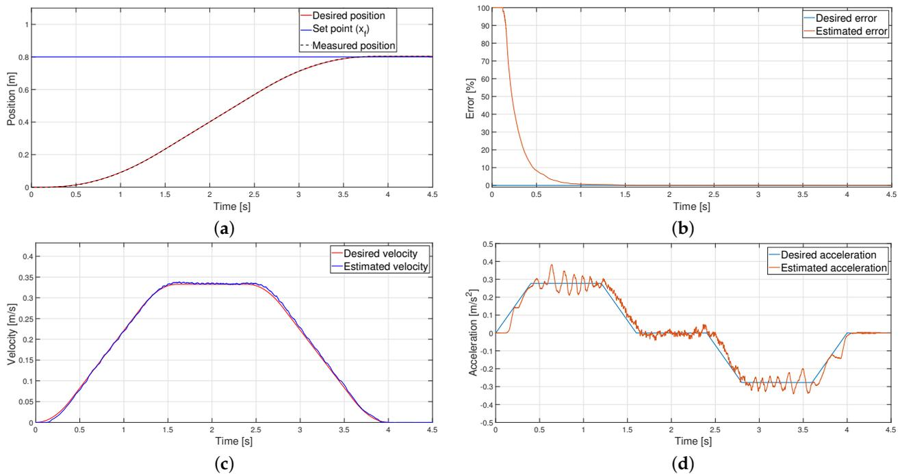
Figure 19. S-curve velocity profile: (a) Position, (b) Error (c) Velocity, and (d) Acceleration.
