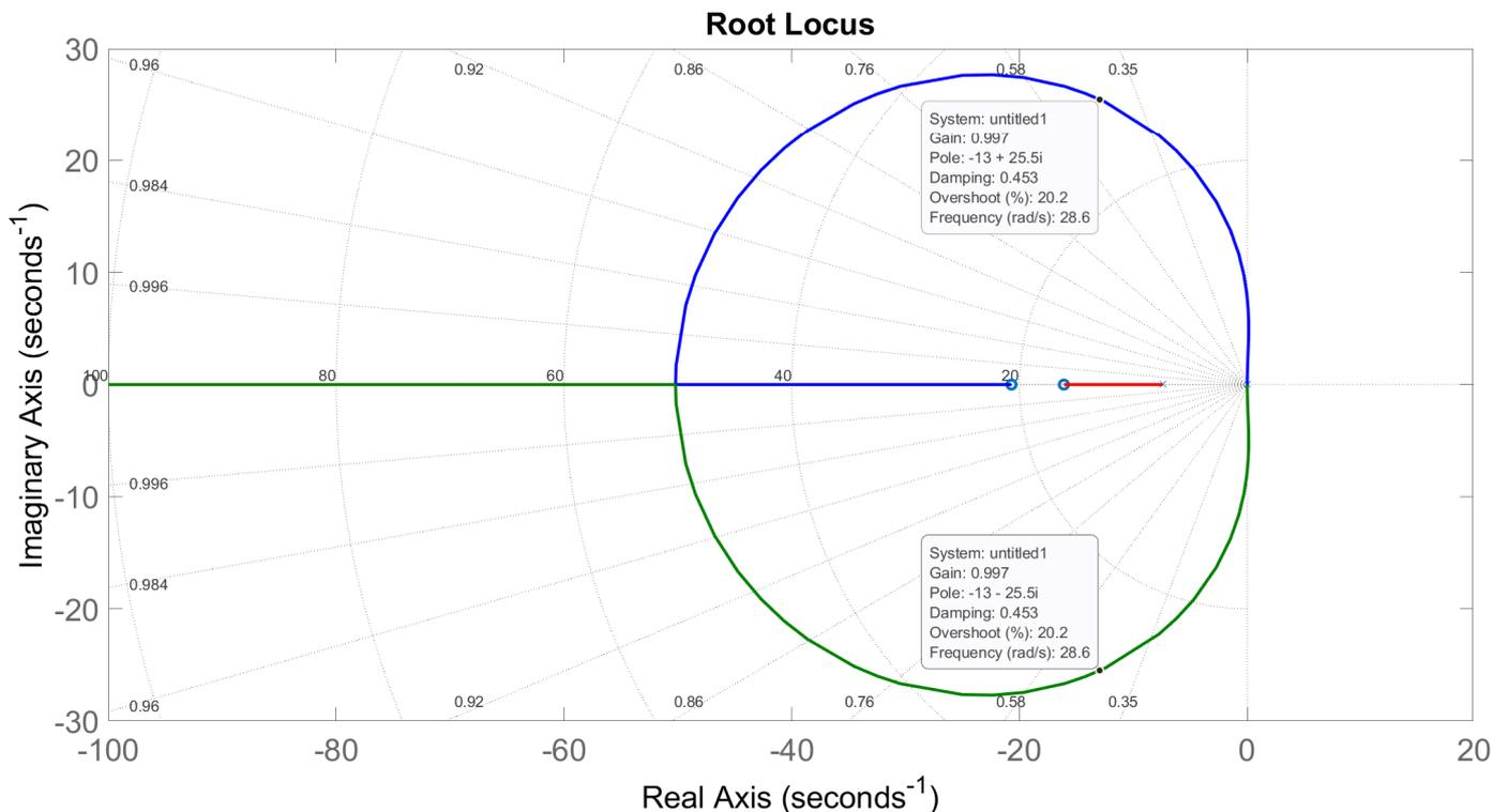
Figure 10. Root Locus of the control system.
