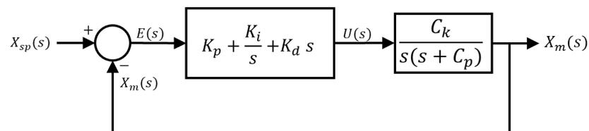
Figure 6. PID algorithm structure.
