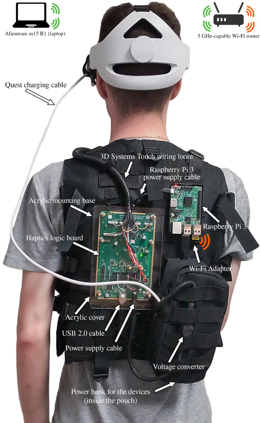
**Figure 4.** System assembly rear view showing the Haptics logic board, as well as the devices enabling wireless communication (Raspberry Pi 3 and a 5-GHz-capable Wi-Fi router), their power source, and the wired connections between Pi 3 and haptics logic board.
