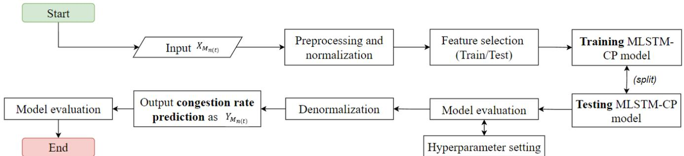
**Figure 3.** Overview of MLSTM-CEFL procedures for denormalizing the hidden state into congestion rate  $Y_{M_{n(t)}}$ .
