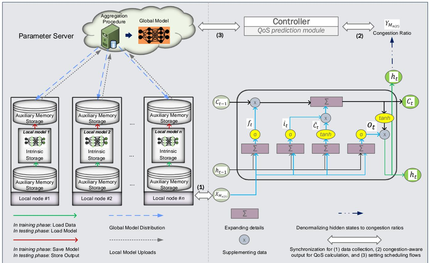
Figure 1. Architecture of IIoT-FL framework with LSTM-based congestion-aware aggregation.
