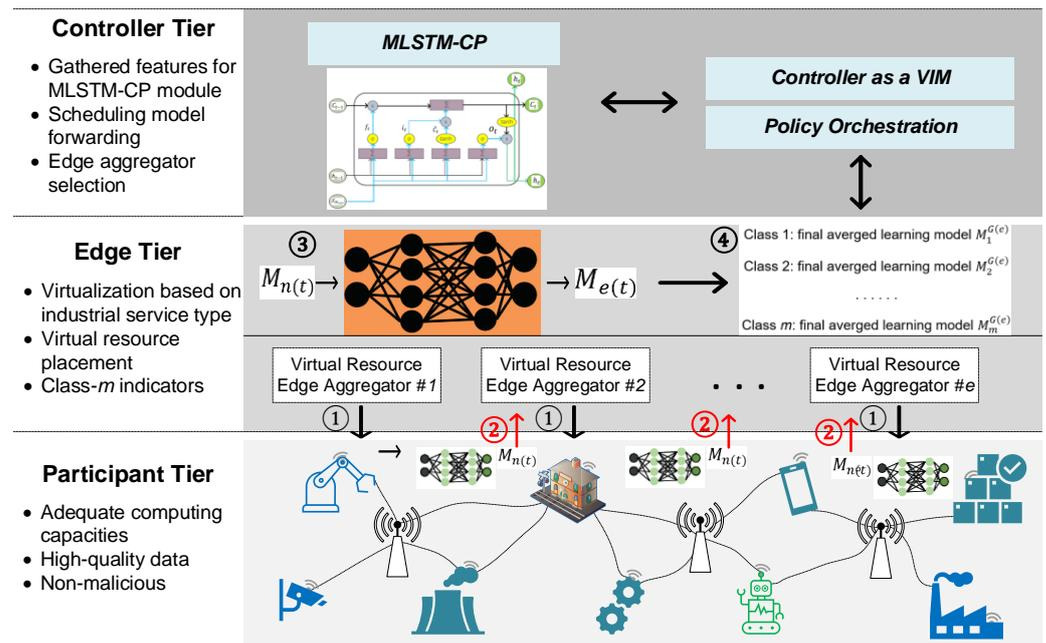
Figure 2. The interactivity of three main tiers in our proposed IIoT-EFL architecture.
