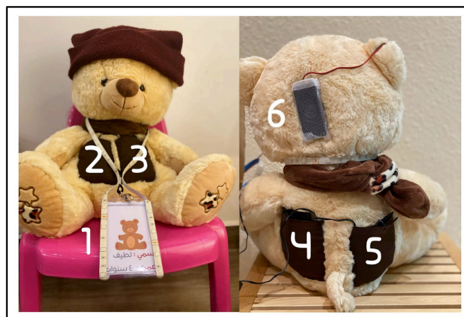
Figure 2. The huggable interface with the light selection (1), heater slices (2–5), and speaker (6).
