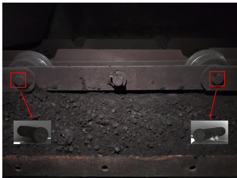
**Figure 1.** The chain is composed of hinge pins and link plates in the metallurgical sites.
