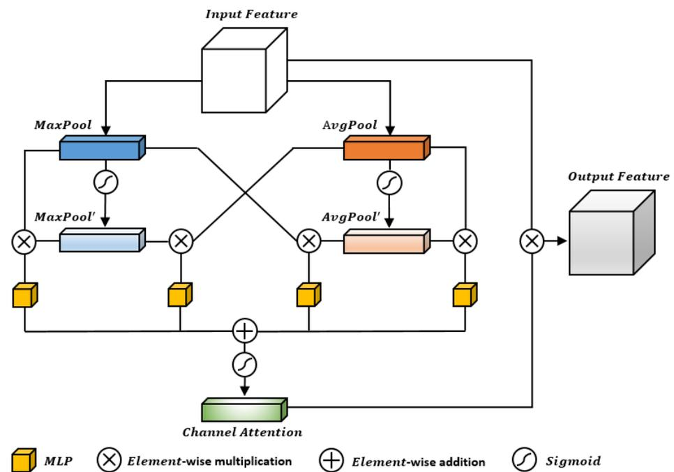
Figure 2. The Cross-Fusion Channel Attention module.
