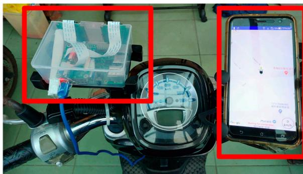
**Figure 17.** Layout of two components of the motorcycle. The left one is the dual-lens device and the right one is the Android phone.
