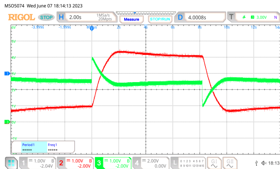
Figure 12. Time waveforms of the PI controller, closed-loop step response of first-order object, e(t) —green, y(t) —red, for x(t) = 0.2 \rightarrow 0.8 , T_i = 3.0 , k_c = 2.0 .
