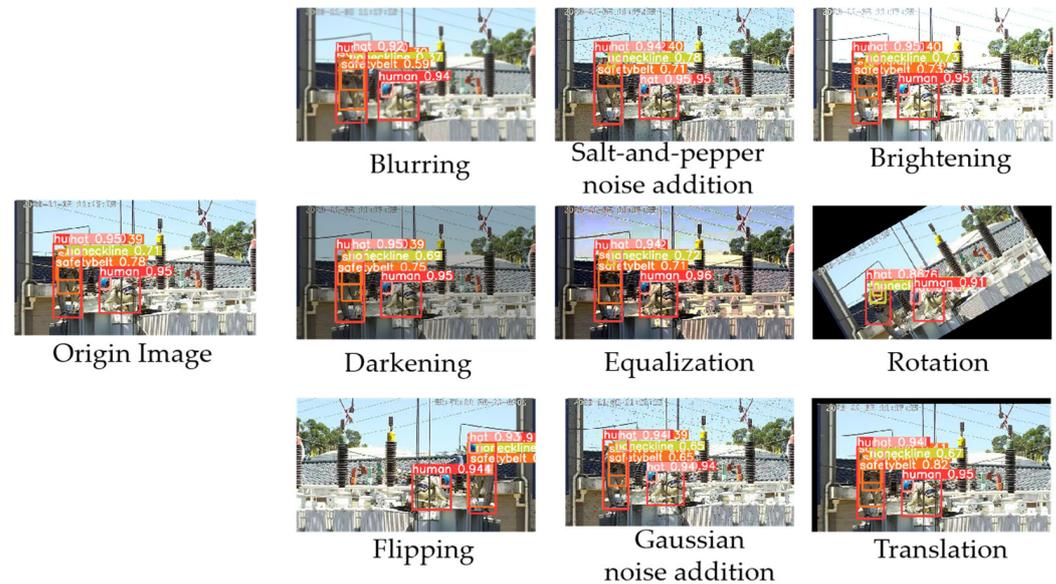
**Figure 12.** The visualization results of images processed using various data augmentation methods.
