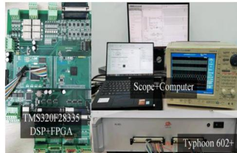
**Figure 18.** Experimental platform of TFSCI based on in-loop control (CHIL).
