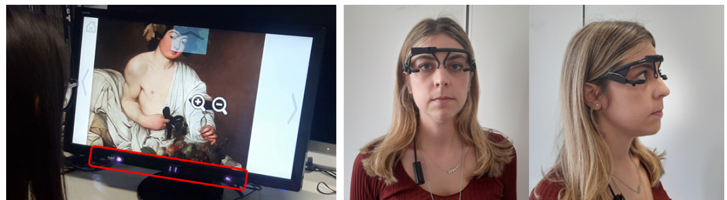
Figure 2. Examples of remote and wearable eye trackers. On the left, highlighted in red, a Tobii 4c (by Tobii) remote device; on the right, a PupilCore (by Pupil Labs) wearable tool — photos taken in our laboratory.
