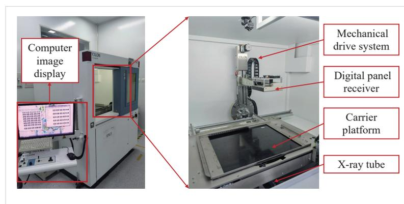
**Figure 1.** X-ray image inspection equipment.
