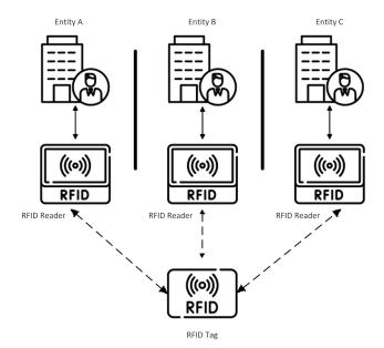
Figure 3. Proposed Port Access Control System.
