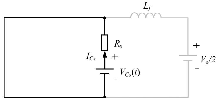
Figure 11. Equivalent circuit of discharge process 2.
