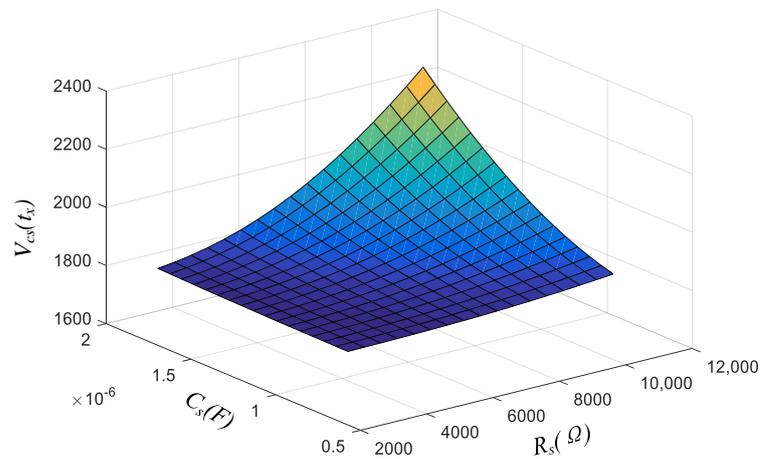
Figure 12. Surface plot of buffer capacitor spike voltage  $V_{C_s}(t_x)$  with  $R_s$  and  $C_s$ .
