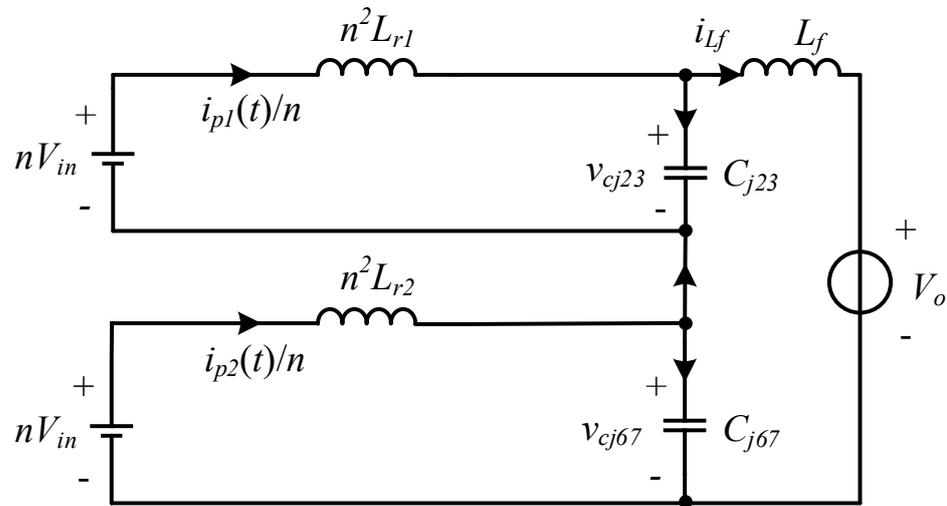
Figure 6. Equivalent circuit for the  $[t_6-t_{10}]$  period.
