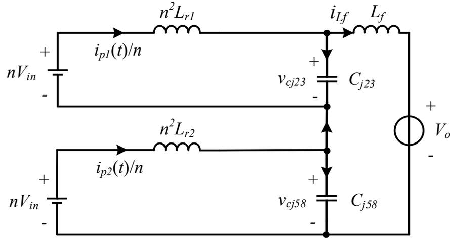
Figure 4. Equivalent circuit for the  $[t_1-t_3]$  period.
