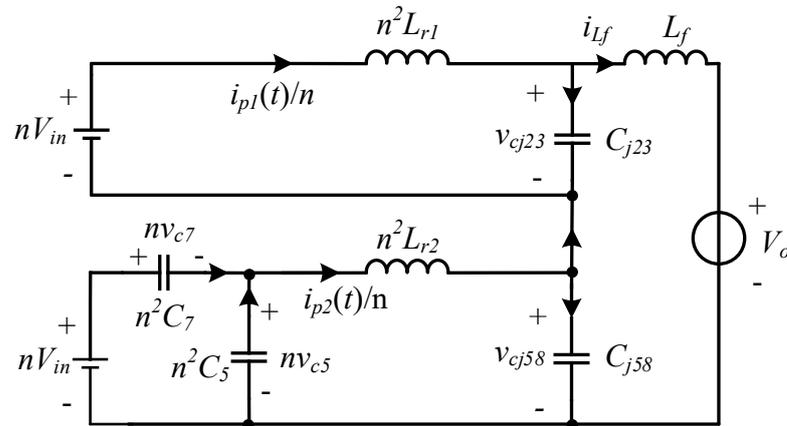
Figure 5. Equivalent circuit for the  $[t_3-t_5]$  period.
