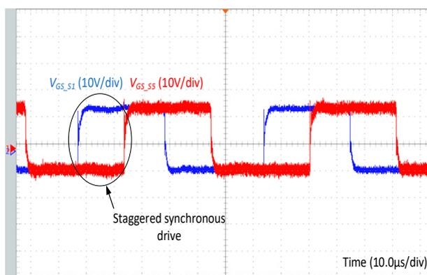
Figure 14. Waveforms of driving pulses of switch transistors  $S_1$  and  $S_5$ .
