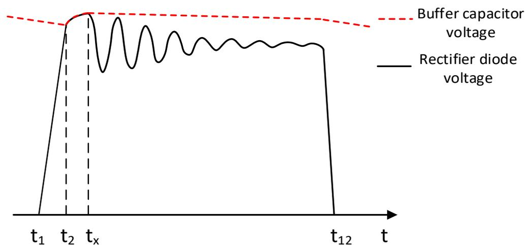
Figure 9. Schematic diagram of diode and buffer capacitor voltages.
