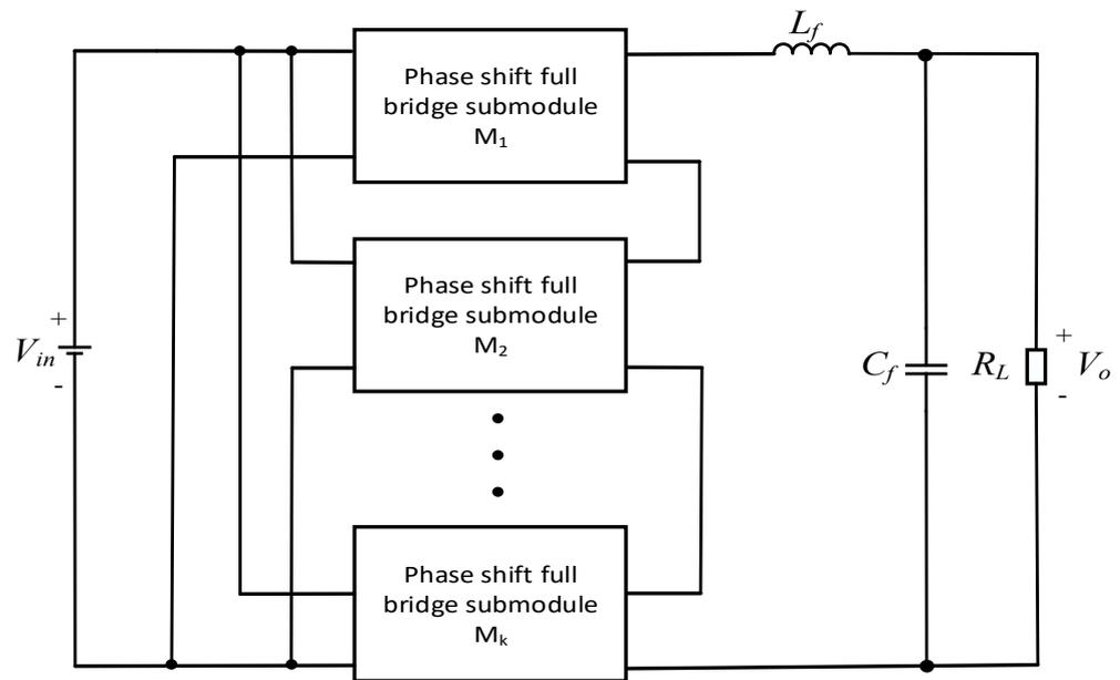
Figure 7. IPOS converter with  $k$  PSFB converter submodules.
