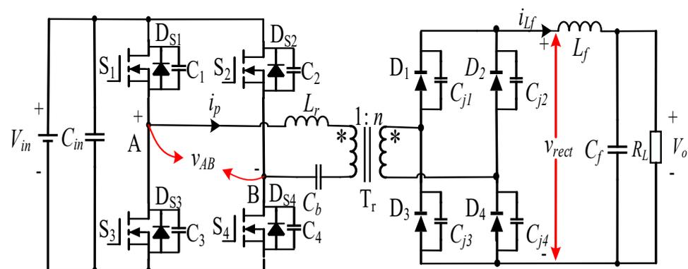
Figure 1. The main circuit of the PSFB converter.
