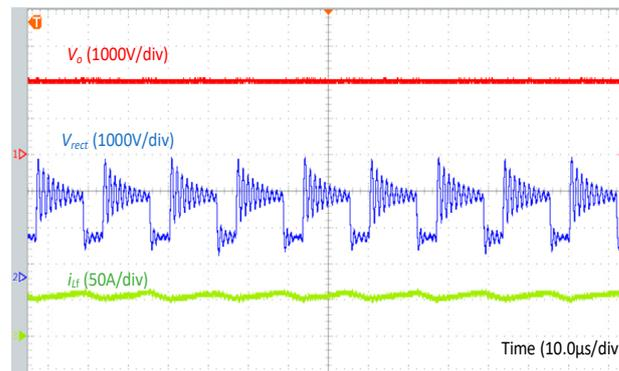
Figure 15. Waveforms of module output voltage  $V_o$ , filter inductor current  $i_{Lf}$  and rectified output voltage  $V_{rect}$ .
