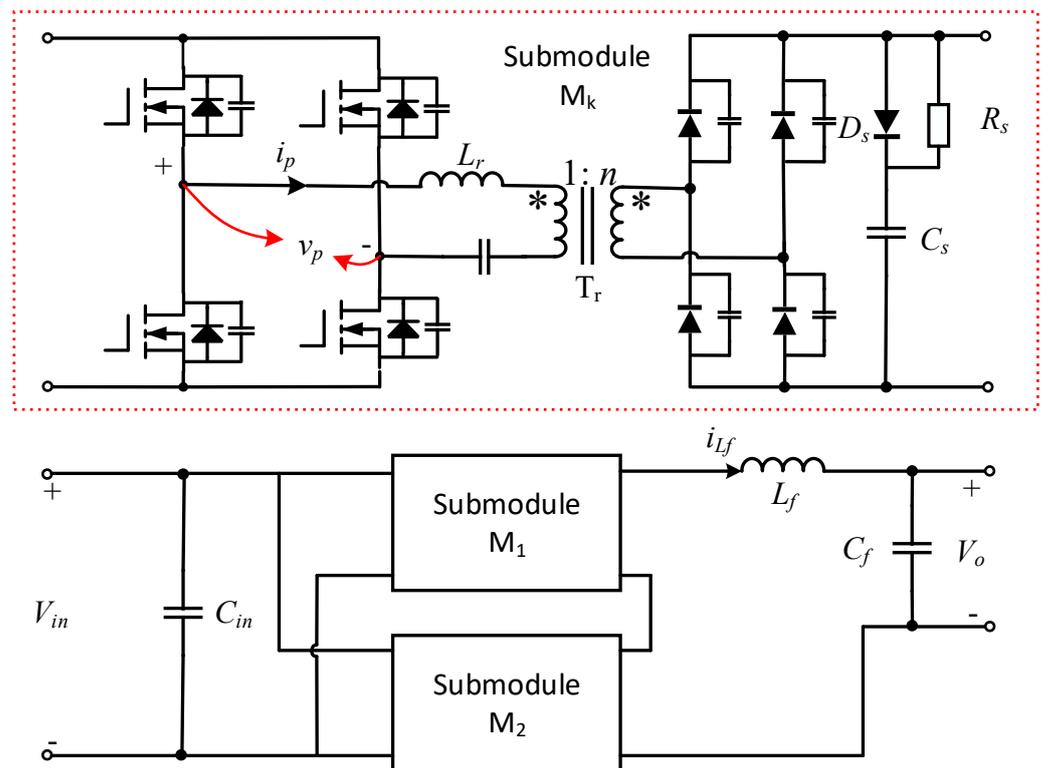
Figure 8. IPOS high-power PSFB converter with RCD buffer circuit.
