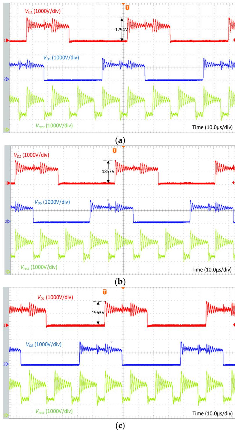
**Figure 18.** Measurement waveforms of rectifier diode spike voltage for different combinations of  $C_s$  and  $R_s$ .
