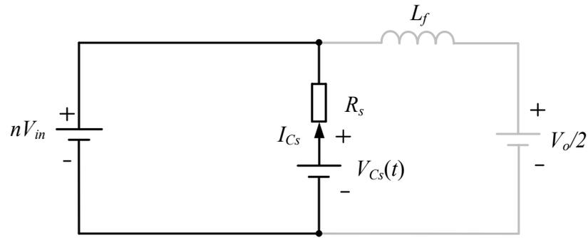
Figure 10. Equivalent circuit of discharge process 1.
