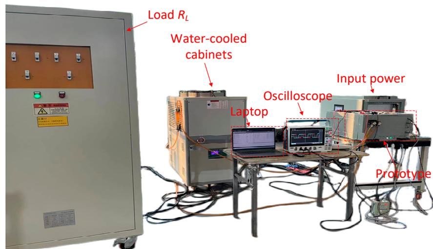
(b) Test stand and measurements
