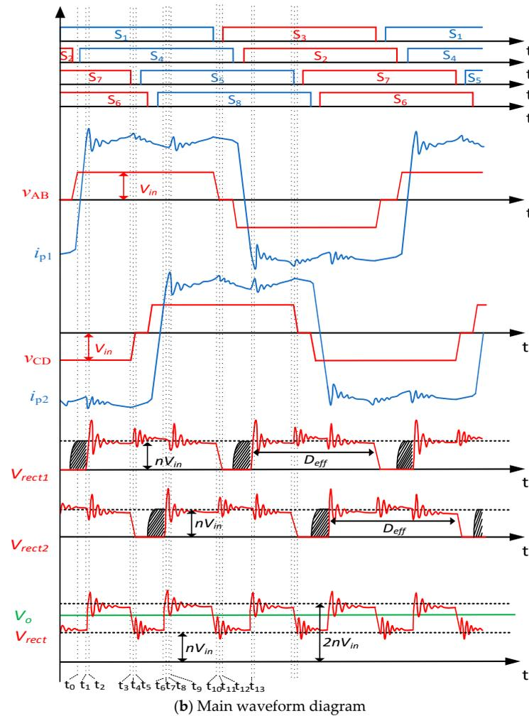
Figure 3. Main circuit and main waveform considering rectifier diode junction capacitance.
