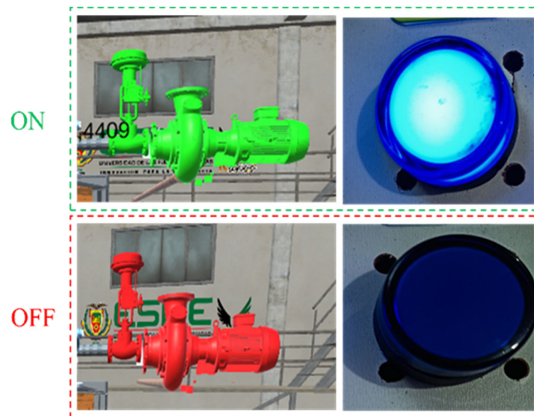
Figure 11. Sample activation of actuators in the virtual work environment vs. indicators on the physical control panel.
