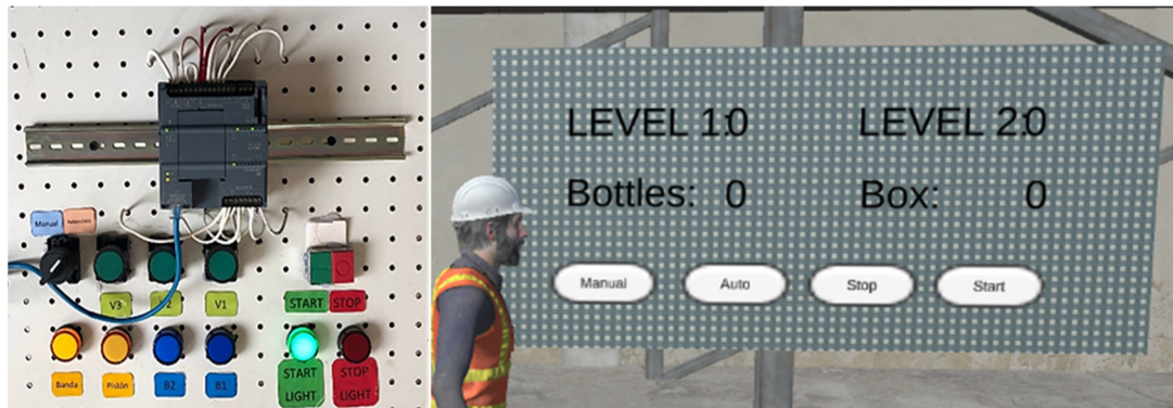
Figure 10. Presentation of physical control panel vs. virtualized control panel.
