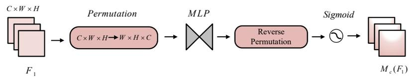
Figure 3. Schematic of channel attention mechanism.
