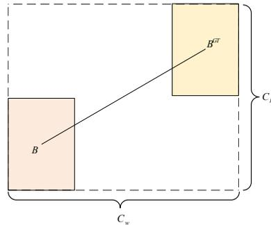
**Figure 9.** Scheme for the distance between the ground truth bounding box and the prediction box.
