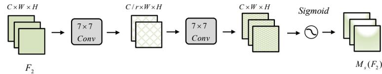
Figure 4. Schematic of spatial attention mechanism.
