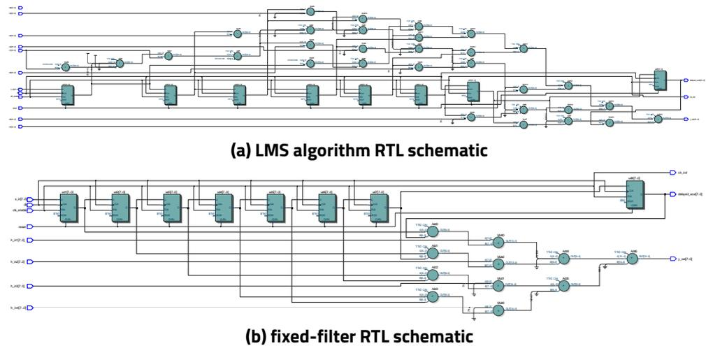
Figure 9. RTL schematics for the (a) LMS algorithm filter and (b) fixed filter.
