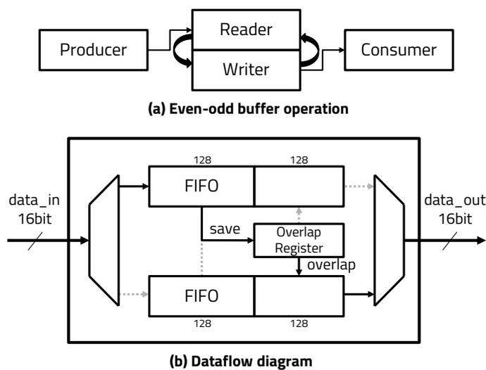
Figure 4. Proposed even–odd buffer structure.
