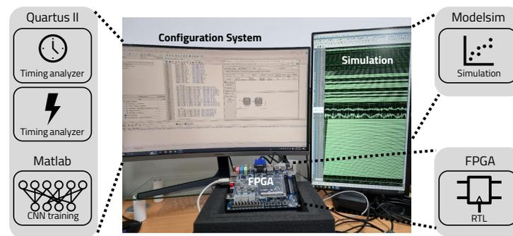
**Figure 6.** Experimental settings with FPGA, configuration system, and simulation.
