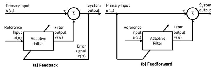
**Figure 1.** Two types of ANC signal processing flow.
