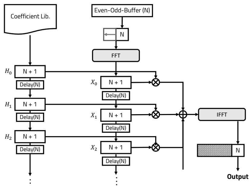
**Figure 5.** Overlap-save method with partitioned convolution.
