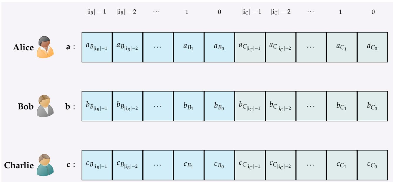
**Figure 7.** This figure gives indicates the contents of Alice, of Bob and Charlie’s input registers after the measurement. The information bit vector  $\mathbf{i}_B$  is revealed by adding (modulo 2)  $\mathbf{a}_B \oplus \mathbf{b}_B \oplus \mathbf{c}_B$ , according to (27). Symmetrically,  $\mathbf{i}_C$  is constructed as  $\mathbf{a}_C \oplus \mathbf{b}_C \oplus \mathbf{c}_C$ , according to (28).
