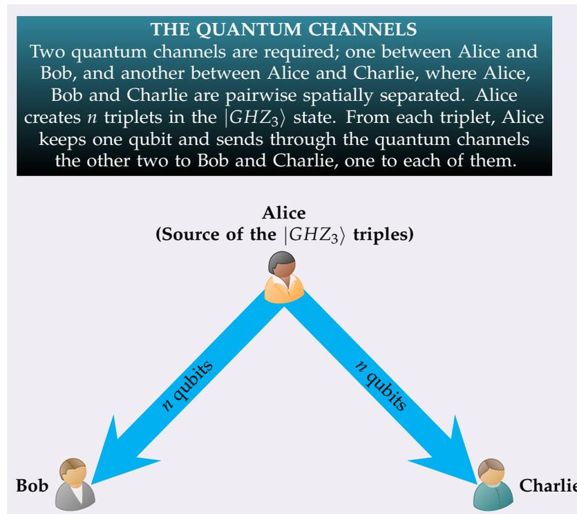
**Figure 4.** This figure shows Alice, Bob and Charlie, who are spatially separated, and the two quantum channels, one between Alice and Bob and the other between Alice and Charlie. Alice produces  $n$  triplets of photons entangled in the  $|GHZ_3\rangle$  state. From each triplet Alice keeps one for herself, sends the second to Bob, and the third to Charlie through the corresponding quantum channels.
