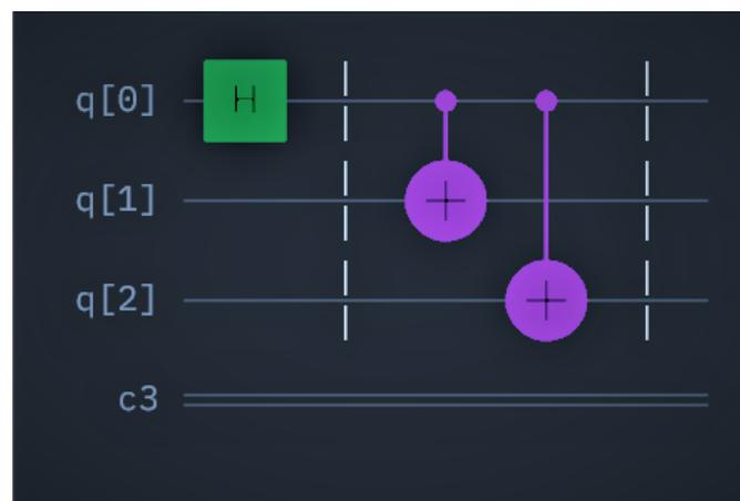
**Figure 1.** The above quantum circuit can entangle 3 qubits in the  $|GHZ_3\rangle = \frac{|0\rangle|0\rangle|0\rangle + |1\rangle|1\rangle|1\rangle}{\sqrt{2}}$  state. Any  $|GHZ_n\rangle$  state can be produced in an analogous manner.
