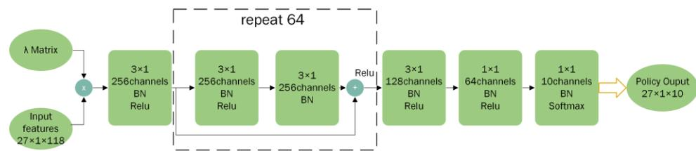
**Figure 5.** The network structure of the normal agent. It uses the product of the observation features and Bernoulli matrix as its input, then, features are extracted through a 64-layer residual block, followed by additional convolutional layers to reduce the dimensionality and establish a direct connection with the policy output.
