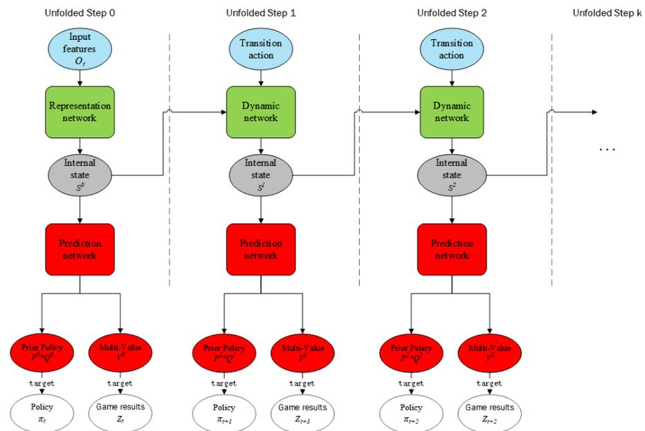
**Figure 4.** The k-step unfolded training process of the learning network. It uses observation features, transition action, and additional transition information as its input, and then outputs prior policy and multi-value for each step.
