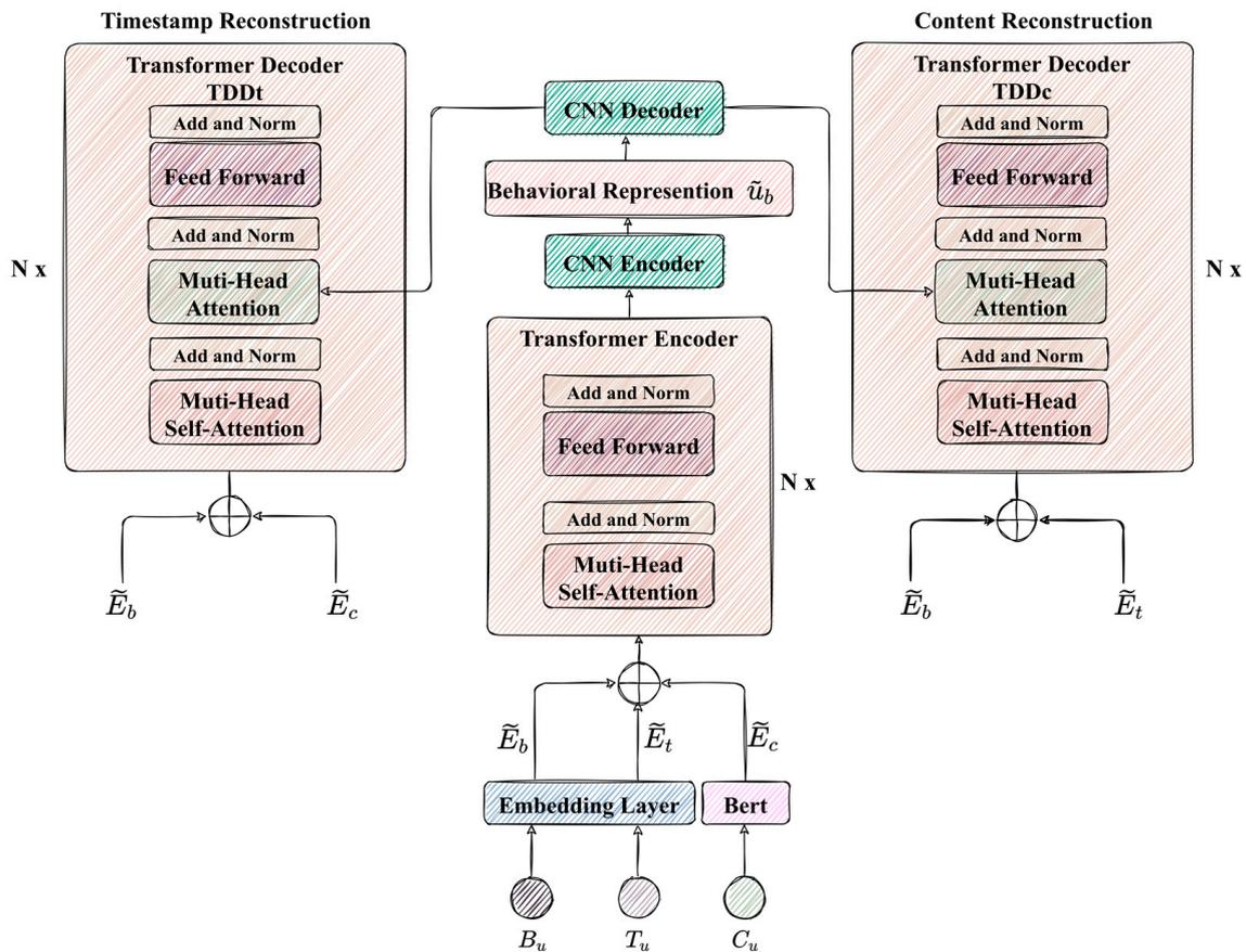
Figure 3. The architecture of DDTCN.
