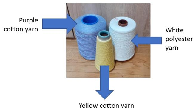
**Figure 35.** Three types of textile yarn tested.
