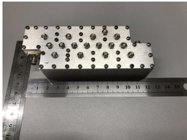
**Figure 9.** Physical view of the new 2080 MHz capacitive-load cavity-filter processed.
