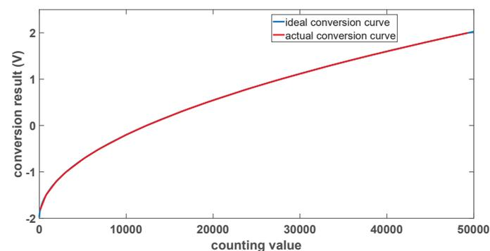
Figure 3. The conversion curve of the memristor-based A/D converter.
