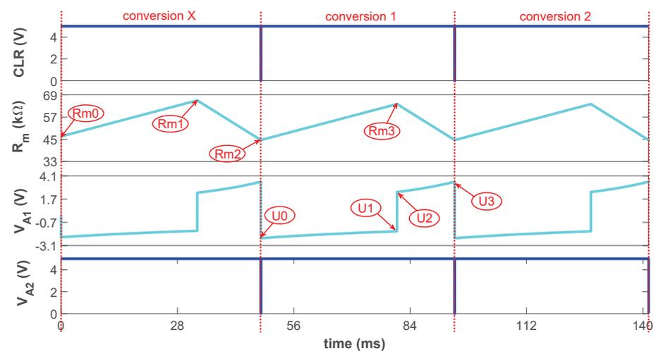
**Figure 2.** The memristance variation and the output voltage change in the fourth simulation.
