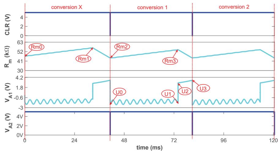
**Figure 4.** The memristance variation and the output voltage change under the input voltage with sine noise.
