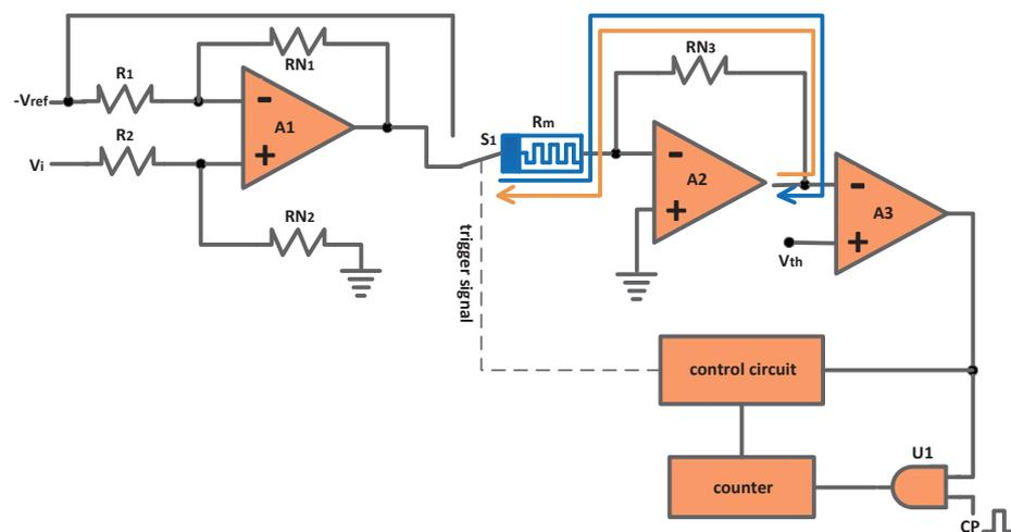
Figure 1. The schematic diagram of the memristor-based A/D converter.
