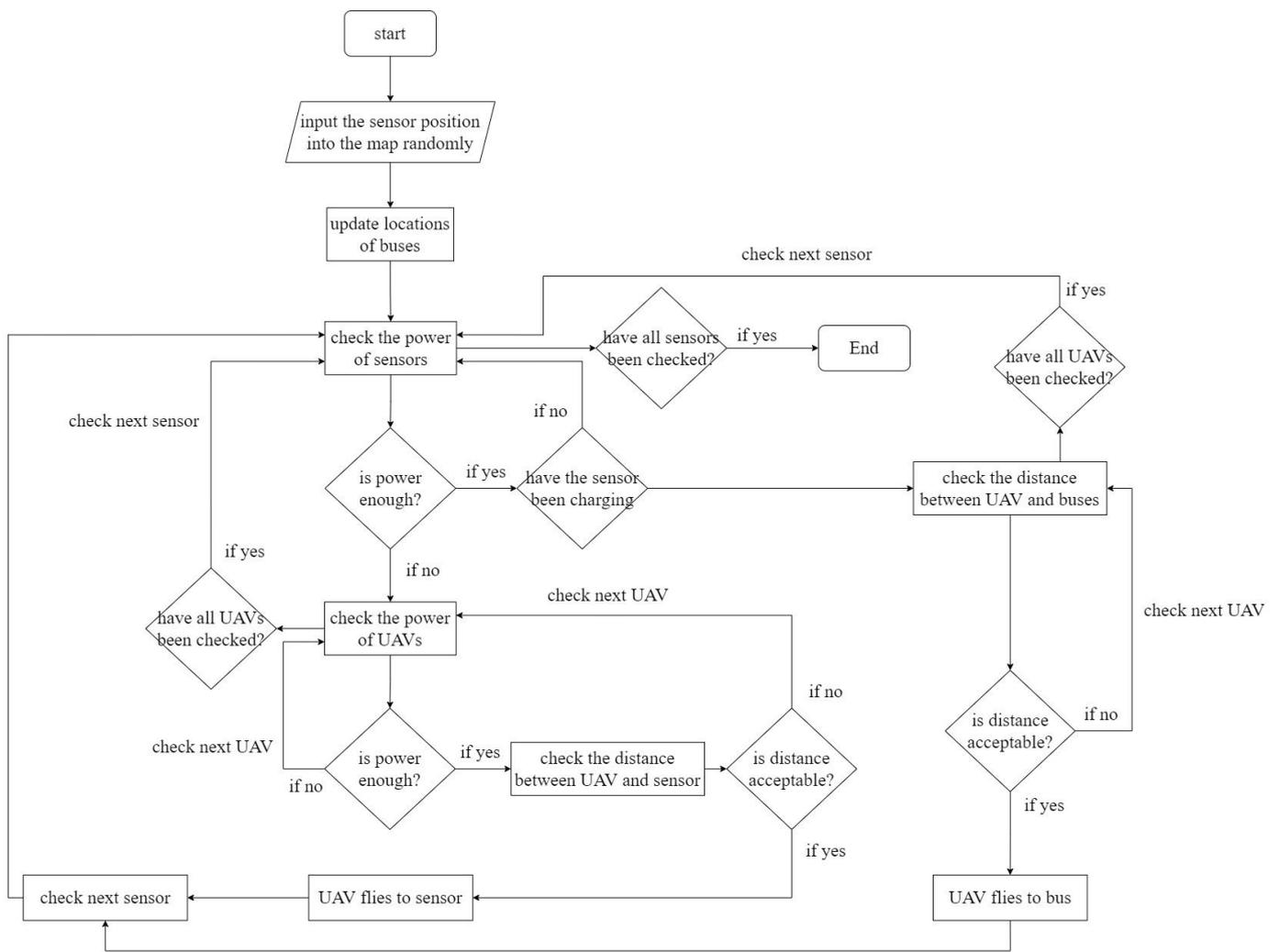
Figure 1. Flow chart of the charging process.
