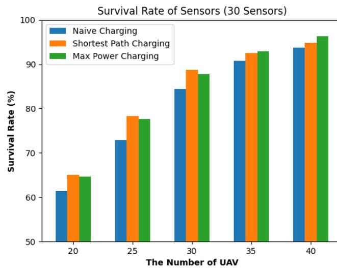
Figure 3. Impact of different algorithms and number of UAVs on the survival rate of sensors.
