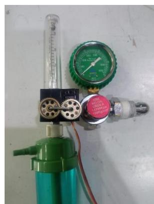
Figure 13. Mechanical implementation in regulator.
