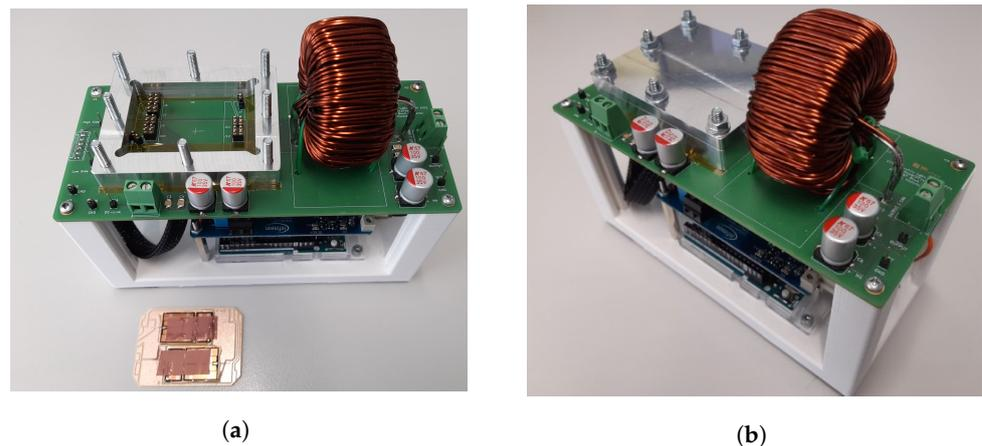
Figure 7. IGBT buck converter hardware photographs with control board (blue) underneath the main power board (green) having bulk energy storage capacitor and inductor components. (a) View with the IGBT-DBC half-bridge removed and not installed on the power board. (b) View with the DBC half-bridge mounted against the spring pressure contacts.
