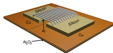
(a) Solid model of a wire-bonded DBC sub-assembly.
