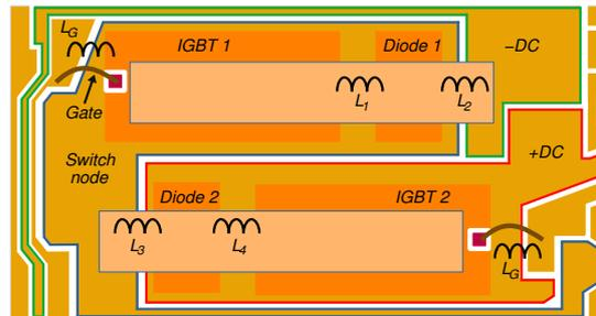
**Figure 2.** Top view of a DBC sub-assembly with Sinterconnects indicating the main parasitic inductances.
