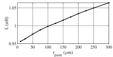
(b) Simulated variation of inductance as a function of copper paste thickness.
