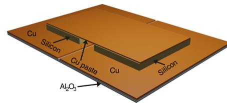
(a) Solid model of a copper-pasted DBC sub-assembly
