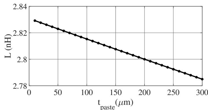
**Figure 3.** Influence of Cu thickness on its equivalent parasitic inductance.
