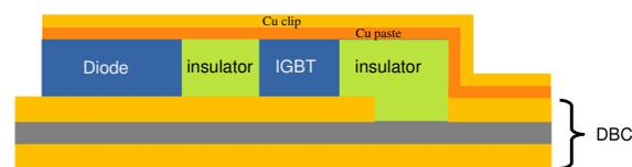
(c) Printed copper-clip attach, cross-sectional view
