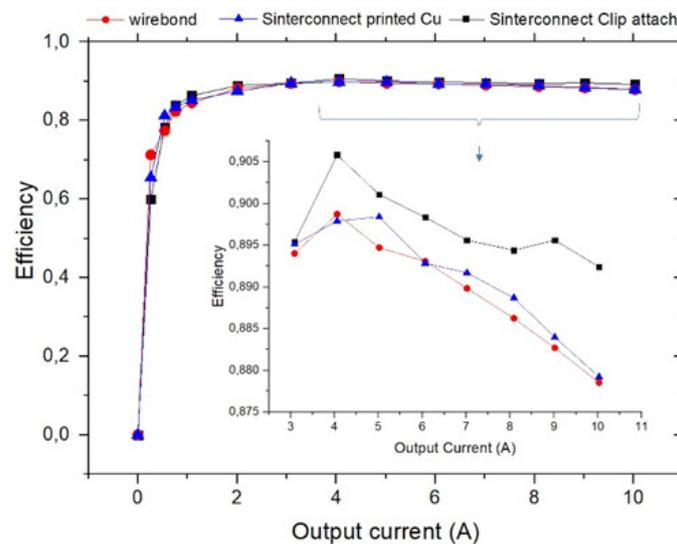
Figure 8. Measured buck converter efficiency values.
