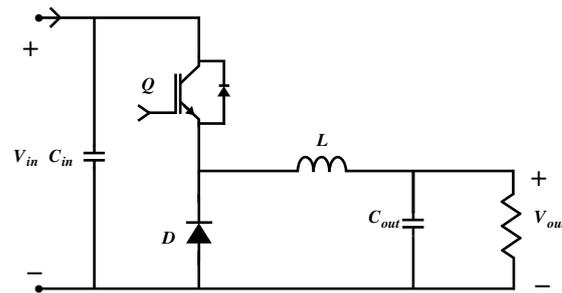
Figure 6. Buck converter schematic.
