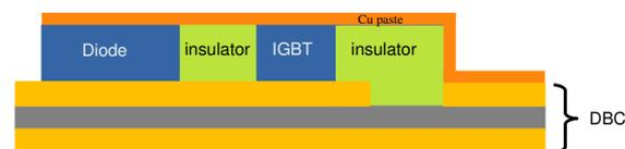
(b) Printed copper-sinter paste, cross-sectional view
