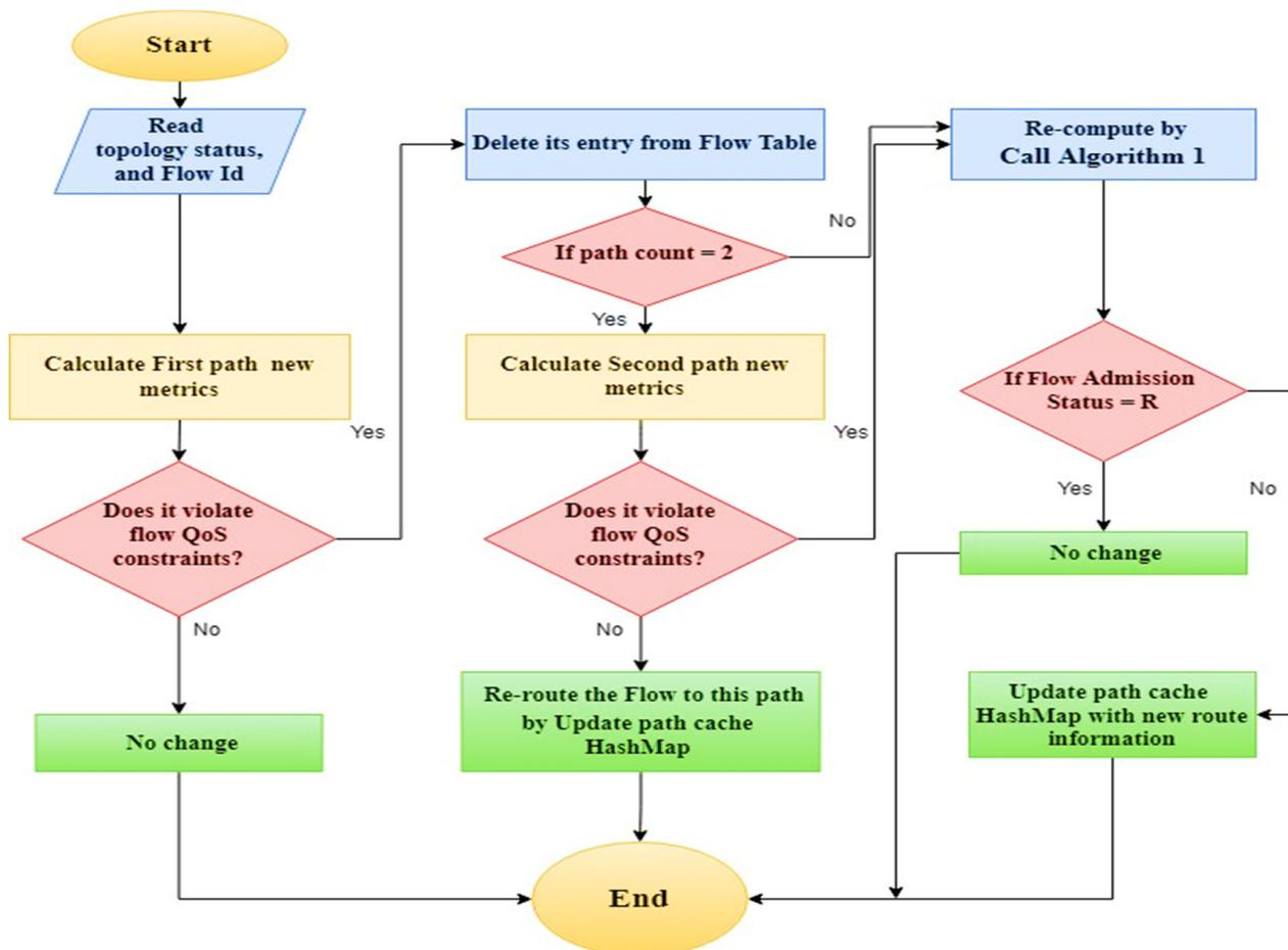
**Figure 2.** Dynamic re-routing algorithm (DR-RA) flowchart.
