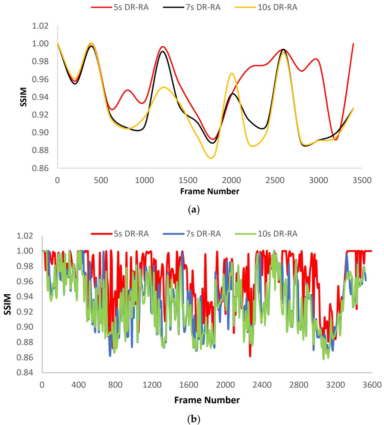
**Figure 8.** Effects of executing dynamic rerouting algorithm at different times in SD video resolution. (a) SSIM values are measured every 10 frames; (b) SSIM values are measured every 200 frames.
