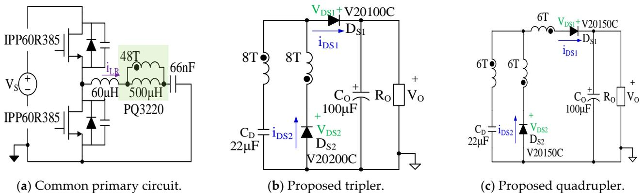
**Figure 5.** Experimental circuits of HB LLC resonant converter.
