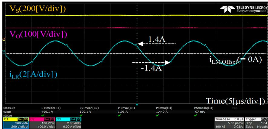
(a) Input voltage ( $V_s$ ), output voltage ( $V_o$ ), and primary resonant transformer current ( $i_{LR}$ ).
