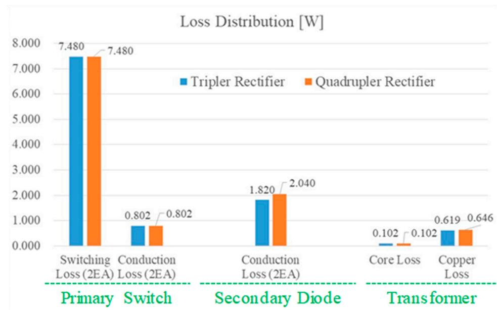
Figure 8. Loss distribution at full-load condition in voltage tripler and quadrupler.
