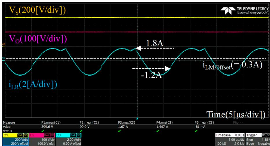
(a) Input voltage ( $V_s$ ), output voltage ( $V_o$ ), and primary resonant transformer current ( $i_{LR}$ ).
