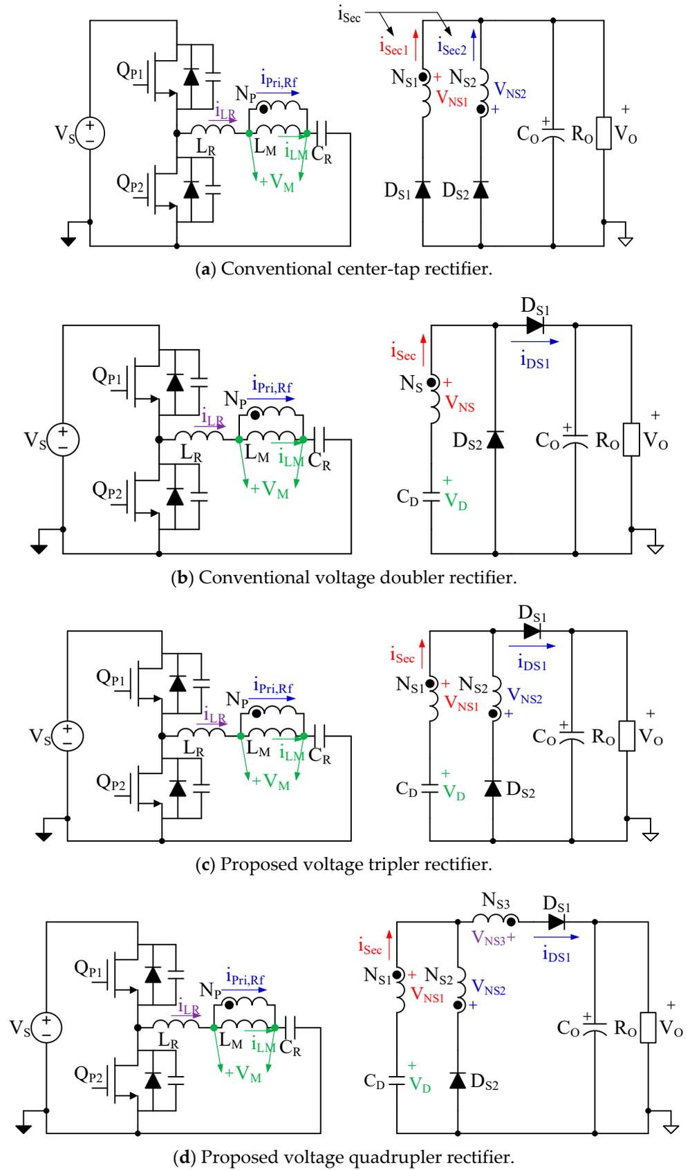
Figure 1. Circuit diagram of conventional and proposed rectifiers.
