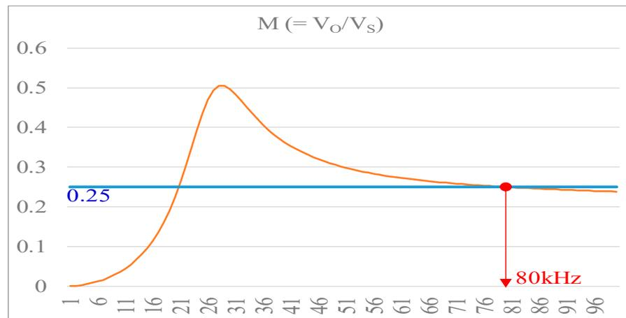
**Figure 4.** Voltage gain (M) of the proposed tripler and quadrupler rectifiers.
