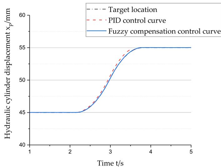
Figure 8. Response curve of the extended position of the hydraulic cylinder.
