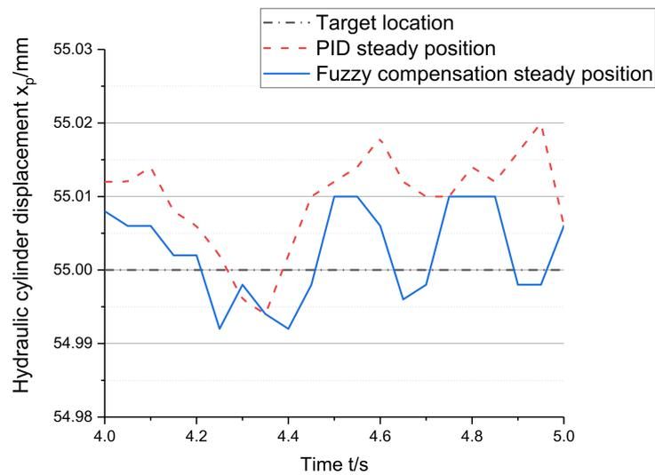
**Figure 9.** Local magnification curve of the extended position of the hydraulic cylinder.
