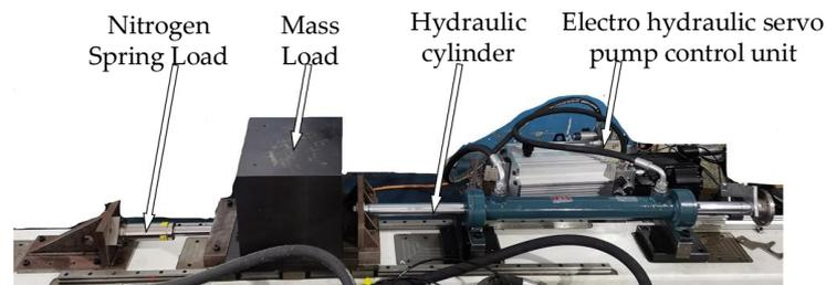
Figure 5. Hydraulic part of experimental platform.
