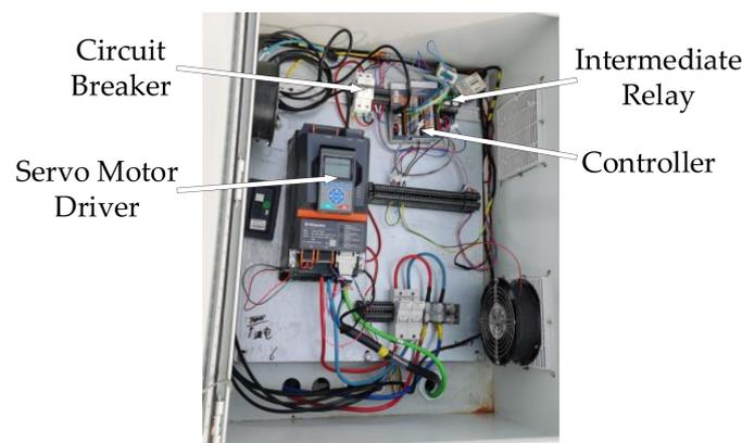
Figure 6. Electrical part of experimental platform.
