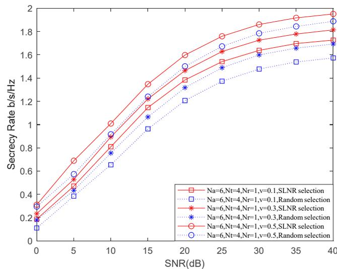
**Figure 2.** SR over SNR under different schemes for different  $v$ .
