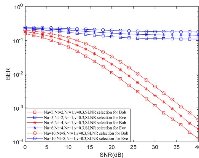
Figure 6. BER over SNR under different schemes for different  $N_a$  and  $N_t$ .
