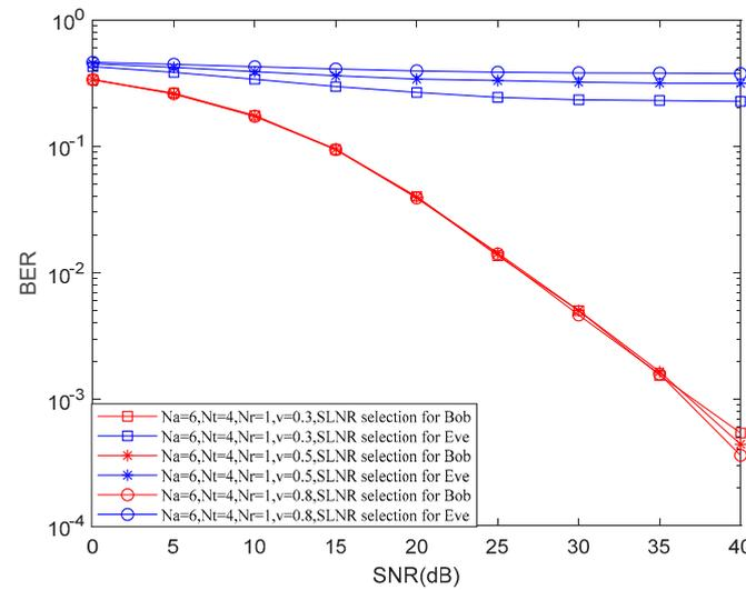
Figure 5. BER over SNR under different schemes for different  $v$ .
