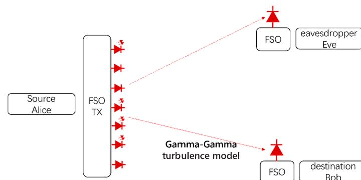
**Figure 1.** System model of SSK-VLC channel.
