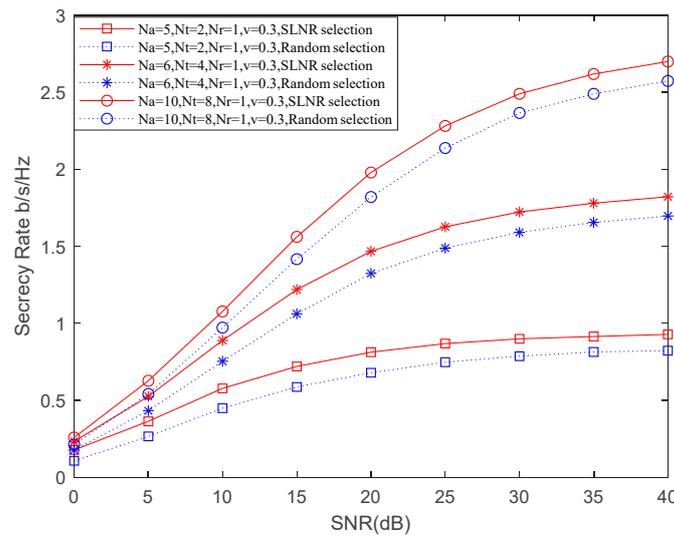
Figure 3. SR over SNR under different schemes for different  $N_a$  and  $N_t$ .
