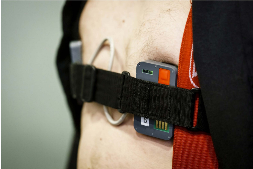
Figure 3. Chest belt of the FlexiGuard monitoring unit used during the study.
