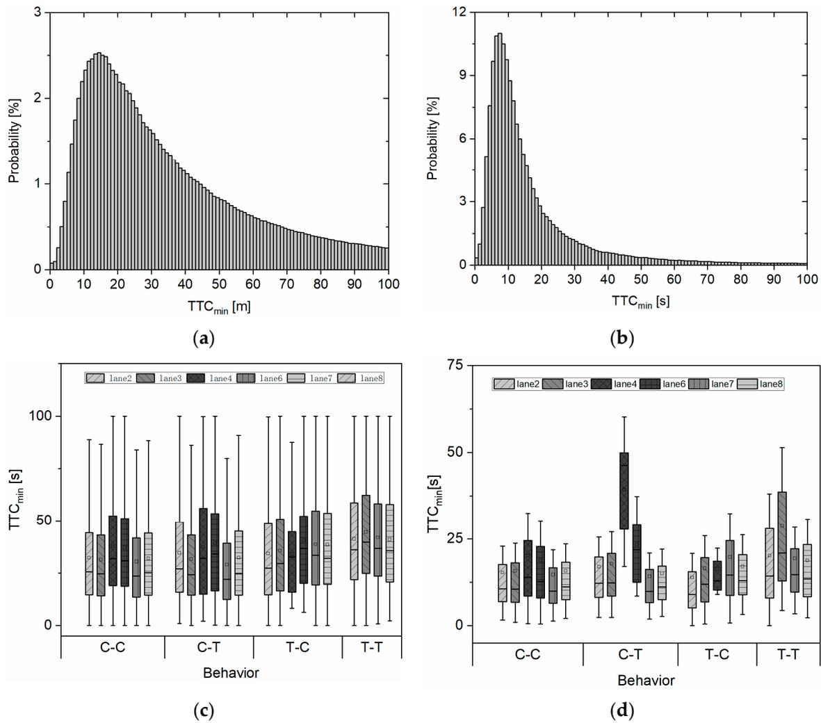
Figure 12. Probability distribution of  $TTC_{min}$  when car following (a) and lane changing (b);  $TTC_{min}$  when car following (c) and lane changing (d) for different following behavior in different lanes.
