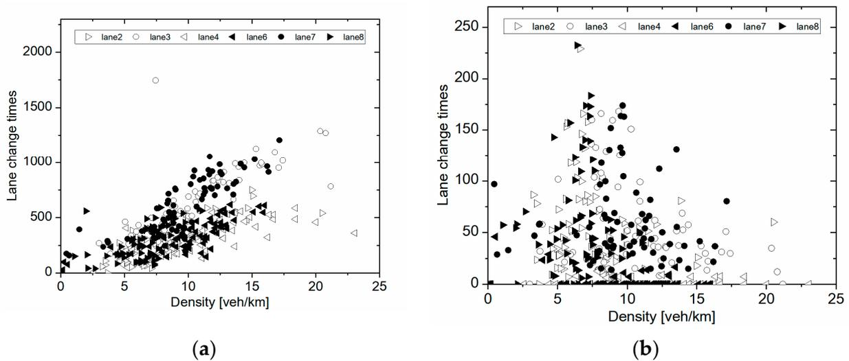
Figure 8. (a) Car lane change times versus density; (b); Truck lane change times versus density.
