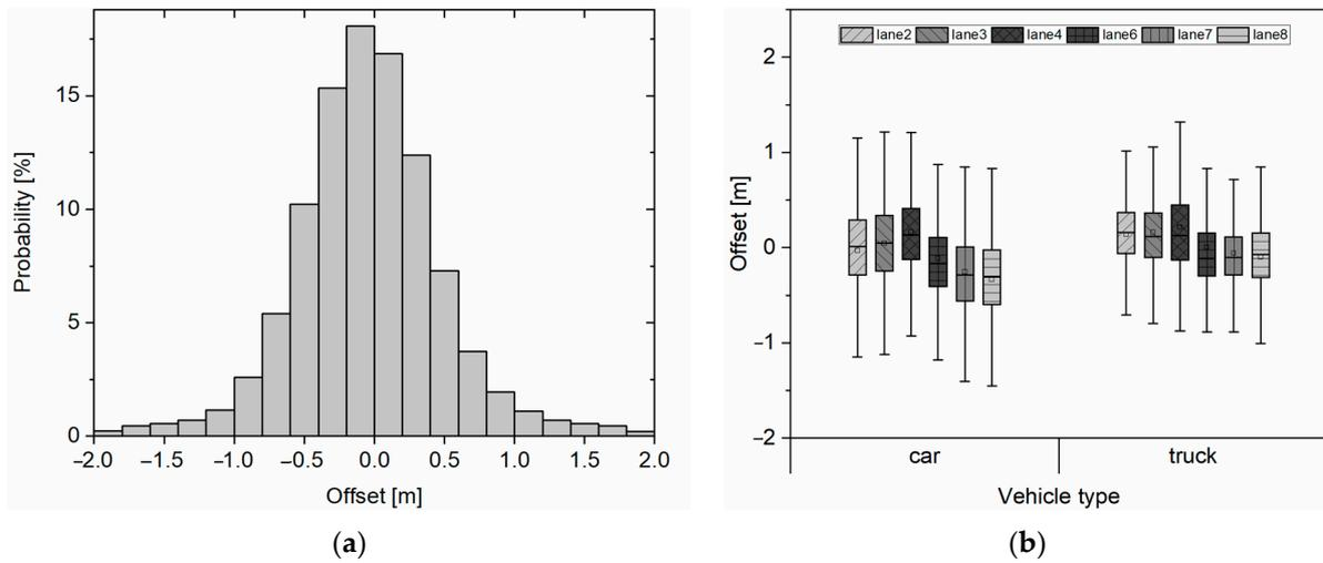
Figure 11. (a) Probability distribution of offset; (b) Offset for car and truck in different lanes.
