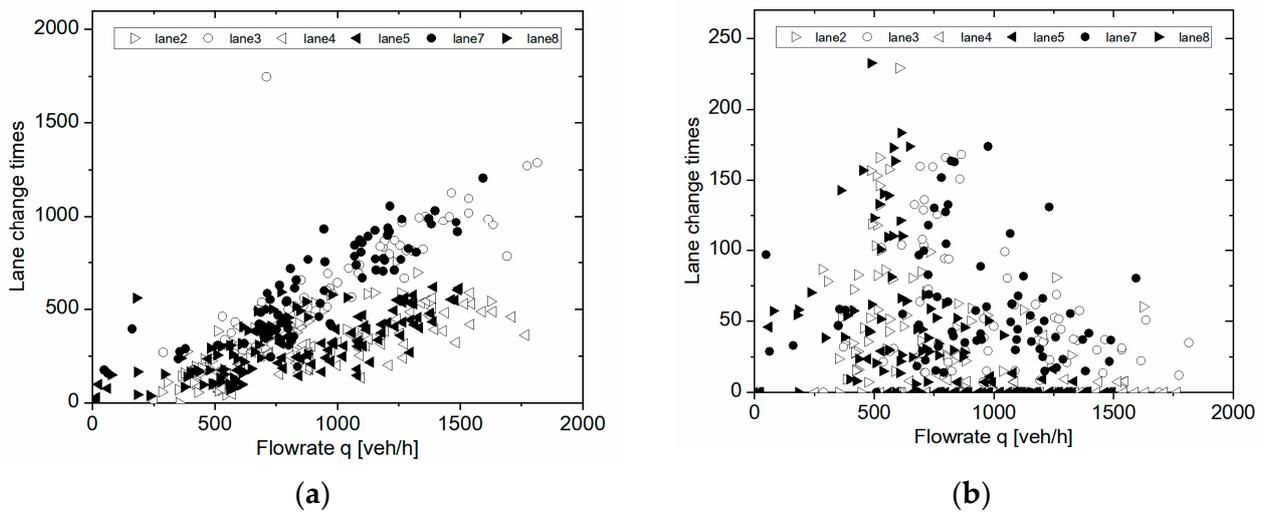
Figure 7. (a) Car lane change times versus flow rate; (b) Truck lane change times versus flow rate.
