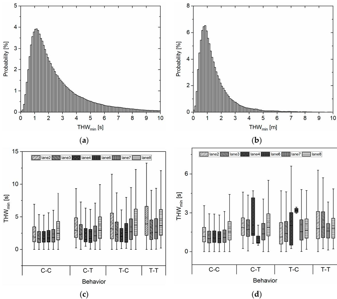
**Figure 13.** Probability distribution of THW<sub>min</sub> when car following (a) and lane changing (b); THW<sub>min</sub> when car following (c) and lane changing (d) for different following behavior in different lanes.
