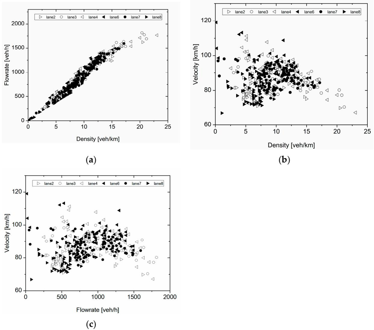
Figure 5. (a) Flow rate versus density; (b) Flow rate versus velocity; (c) Velocity versus density.
