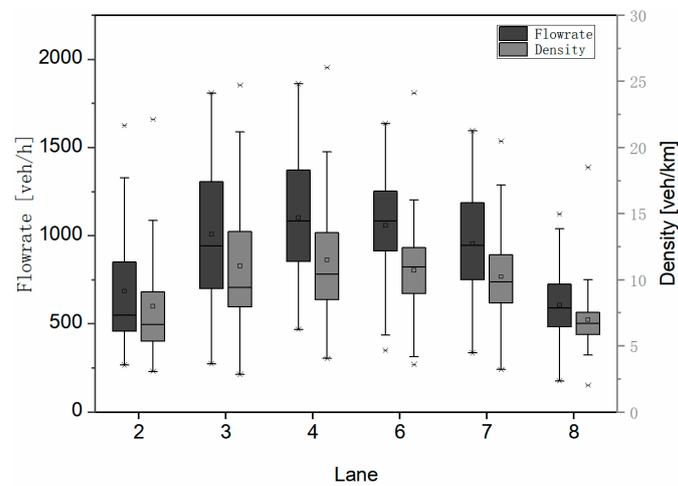
Figure 6. Flow rate and density in different lanes.
