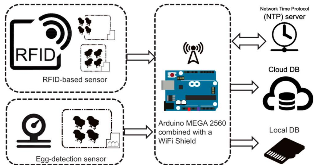
**Figure 16.** Block diagram of IoT platform for poultry-laying performance and behavior monitoring [70].
