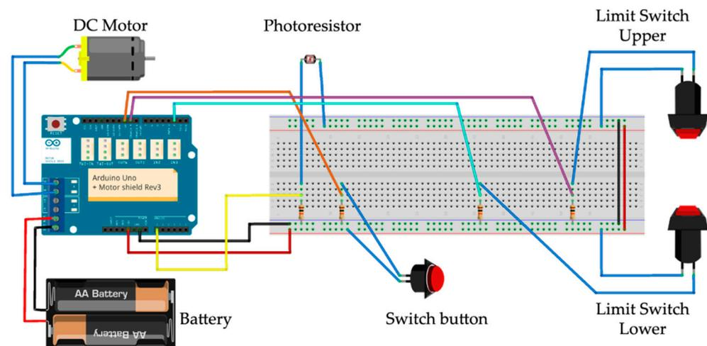
Figure 17. Arduino-based smart chicken coop door, DIY project [72].
