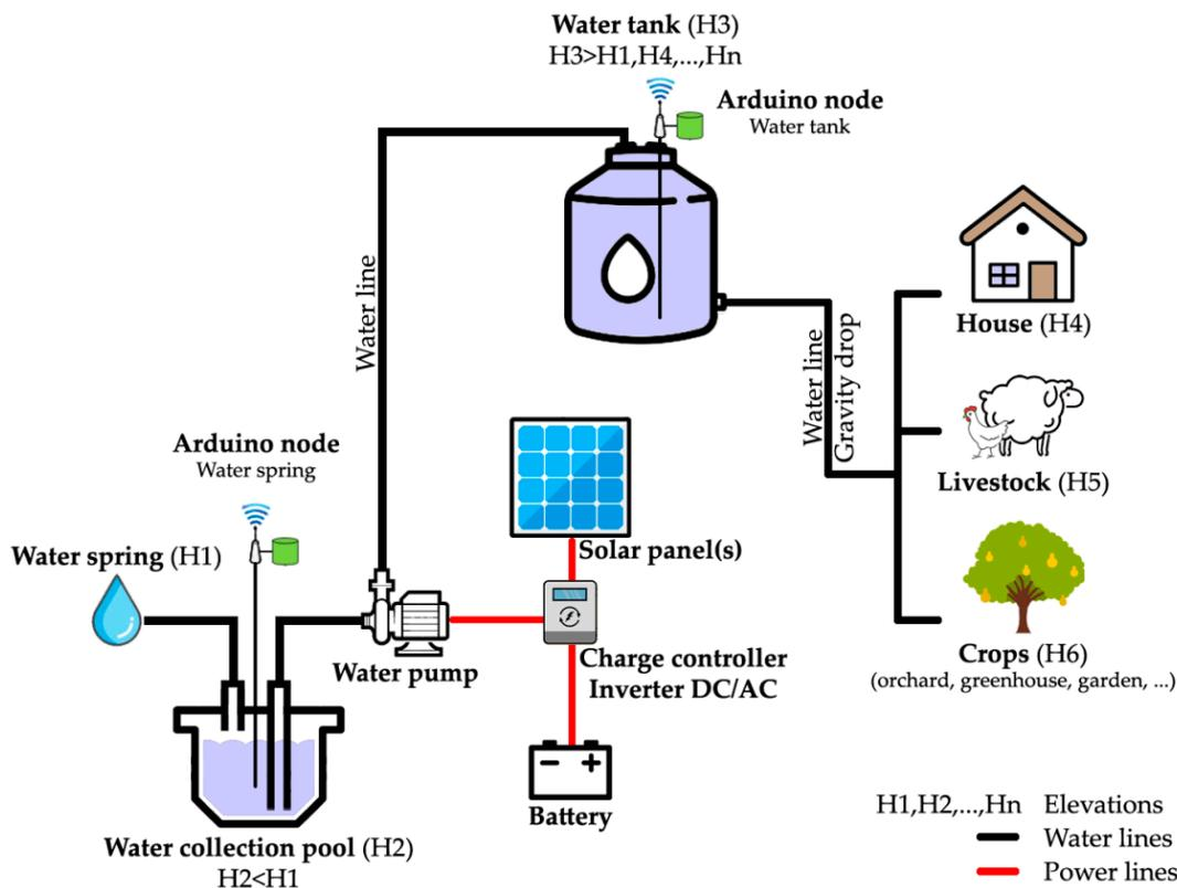
Figure 9. Autonomous wireless water management system in mountainous homestead.
