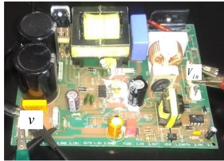
Figure 6. The experimental setup of boost converter.
