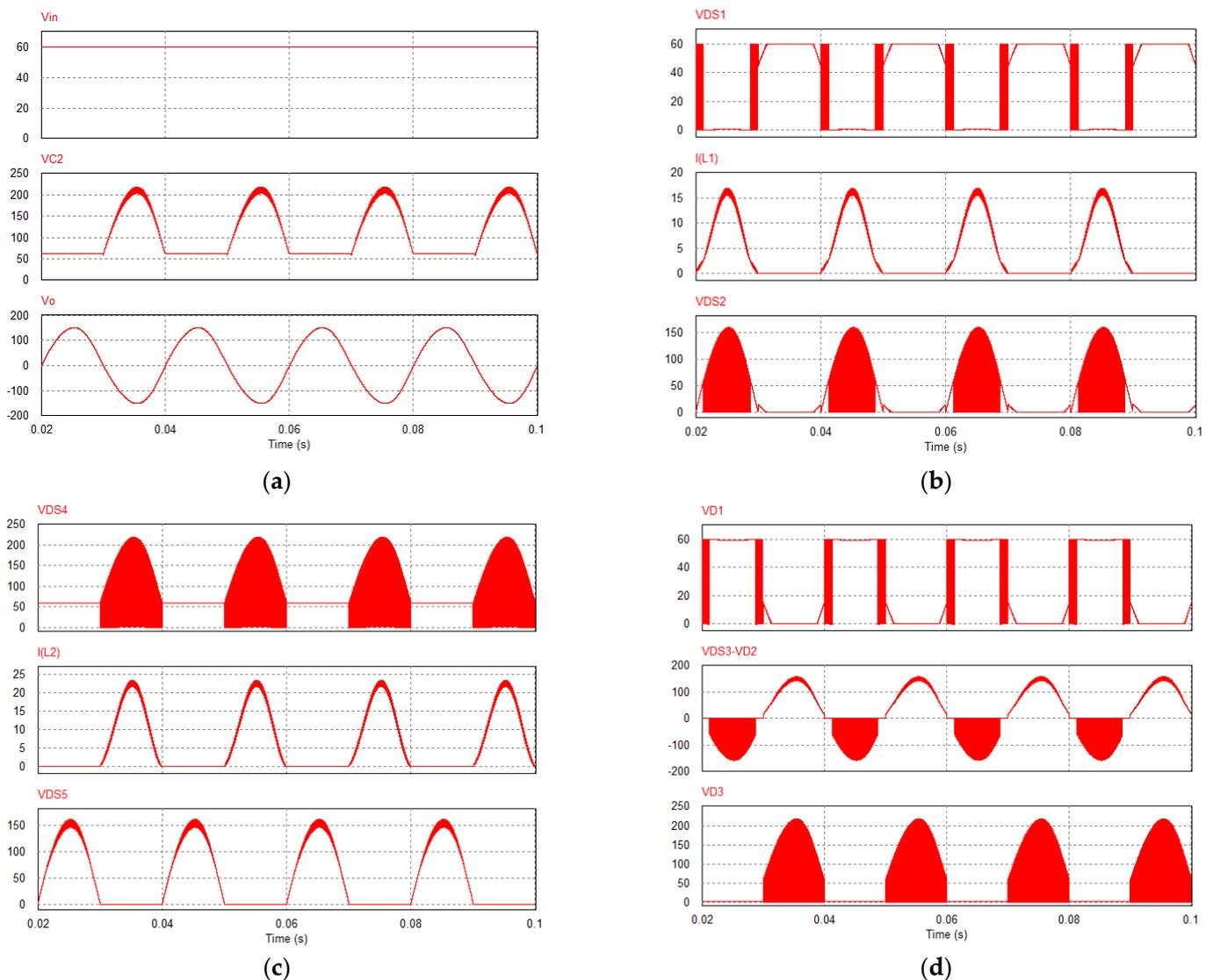
**Figure 6.** Simulation results with  $V_{in} = 60$  V: (a) the input, output and capacitor  $C_2$  voltages, (b) the voltage stress on switches  $S_1$ ,  $S_2$ , and the current of inductor  $L_1$ , (c) the voltage stress on switches  $S_4$ ,  $S_5$ , and the current of inductor  $L_2$ , and (d) the voltage stress on diodes  $D_1$ ,  $D_2$ ,  $D_3$  and the voltage stress on switch  $S_3$ .
