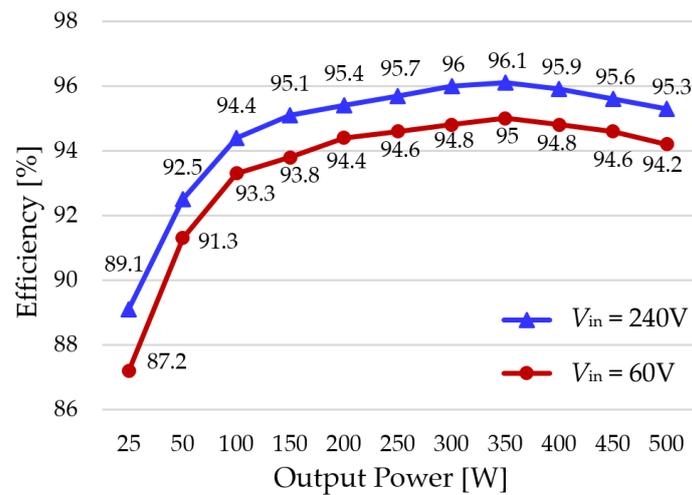
Figure 10. Efficiency measurement with  $V_{in} = 60 V$  and  $V_{in} = 240 V$ .
