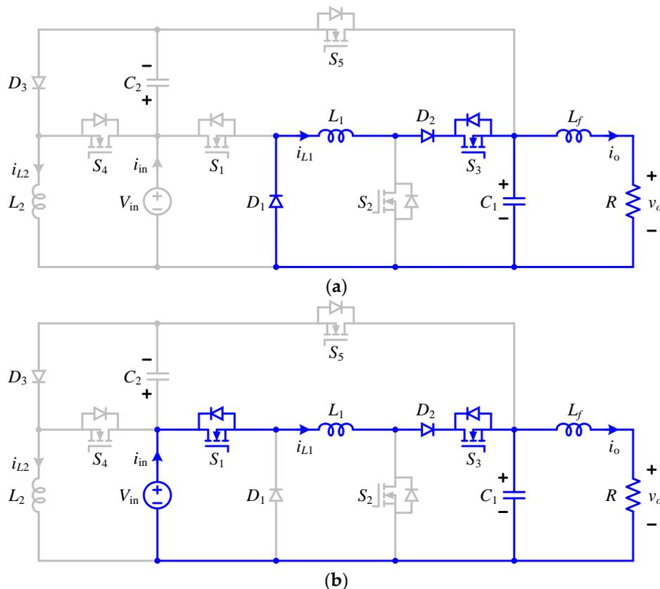
**Figure 3.** Equivalent circuits of the proposed CGBBI topology in interval 1 when  $0 < v_o < V_{in}$ : (a) mode 1 and (b) mode 2.
