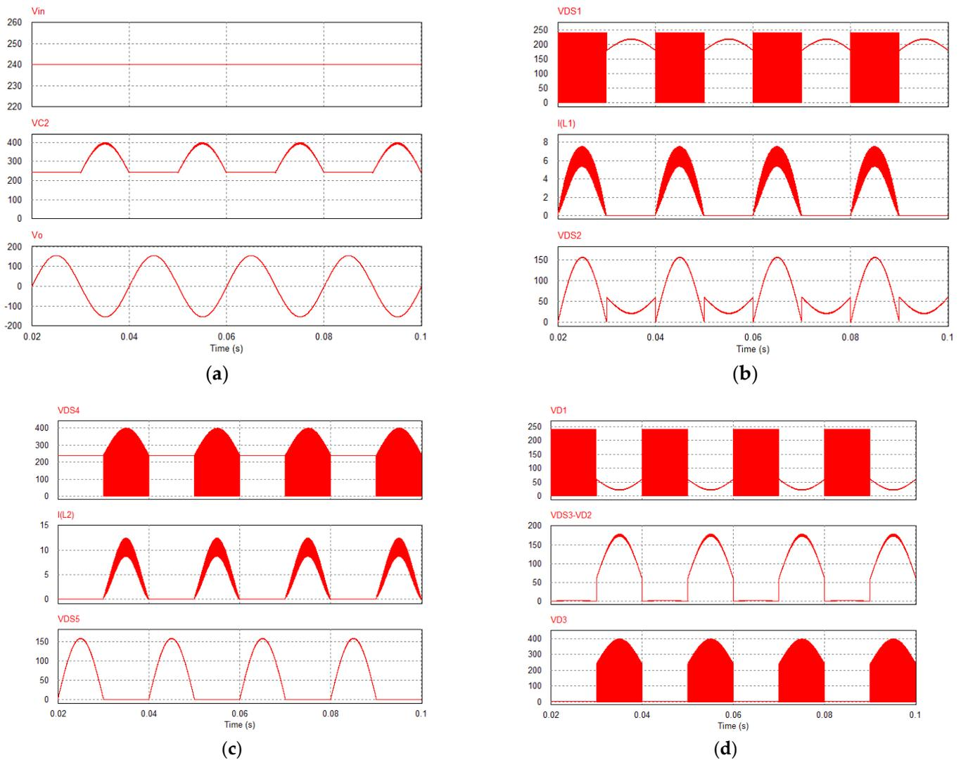
**Figure 7.** Simulation results with  $V_{in} = 240$  V. (a) the input, output and capacitor  $C_2$  voltages, (b) the voltage stress on switches  $S_1, S_2$ , and the current of inductor  $L_1$ , (c) the voltage stress on switches  $S_4, S_5$ , and the current of inductor  $L_2$ , and (d) the voltage stress on diodes  $D_1, D_2, D_3$  and the voltage stress on switch  $S_3$ .
