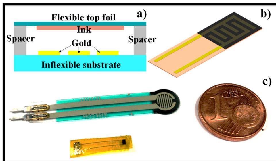
**Figure 6.** (a) Cross-sectional view of a force-sensing resistor. Inspired by the work in [132], (b) render image of a sensing instrument design proposed in [131]. (c) Photography of the sensing instrument design proposed in [131] (**bottom left**), and an FSR by Interlink (**top left**).
