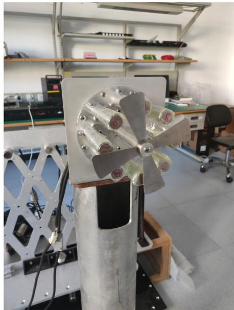
Figure 7. The rotating shutter antenna.
