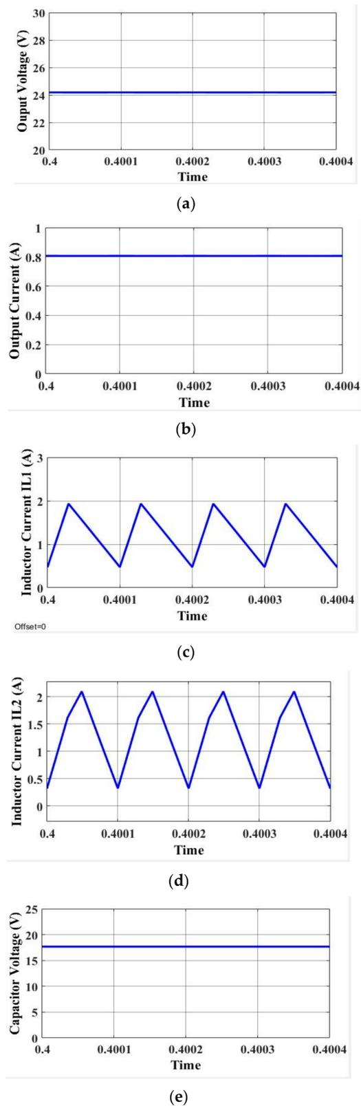
**Figure 7.** Output wave forms of step-down mode. (a) Output voltage, (b) output current, (c) inductor current ( $I_{L1}$ ), (d) inductor current ( $I_{L2}$ ), and (e) capacitor voltage ( $V_{C1}$ ).
