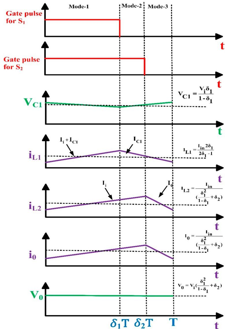
Figure 2. The proposed converter’s waveforms for one switching interval.
