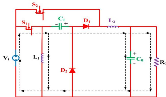
Figure 1. Proposed hybrid Zeta converter.
