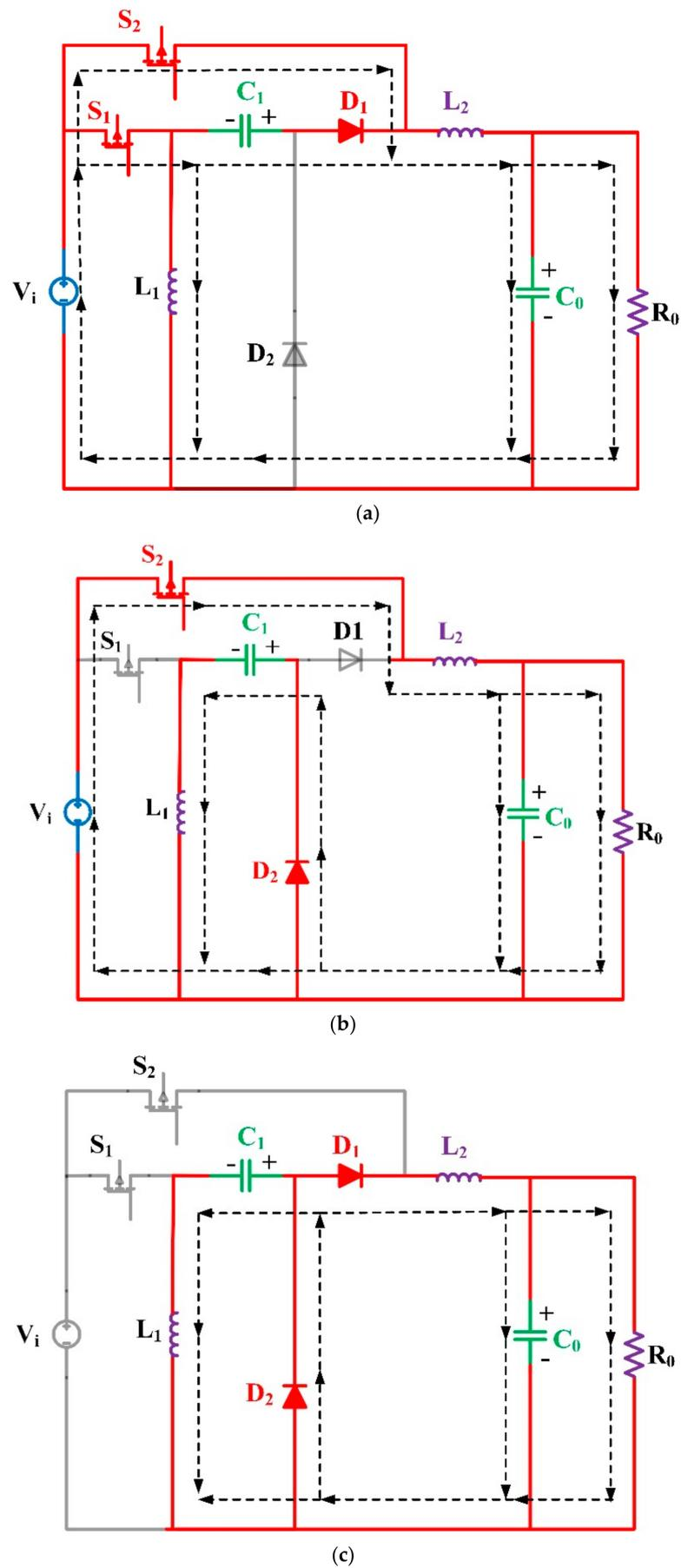
Figure 3. The proposed hybrid Zeta converter equivalent circuits. (a) Mode-1 (b) Mode-2 (c) Mode-3.
