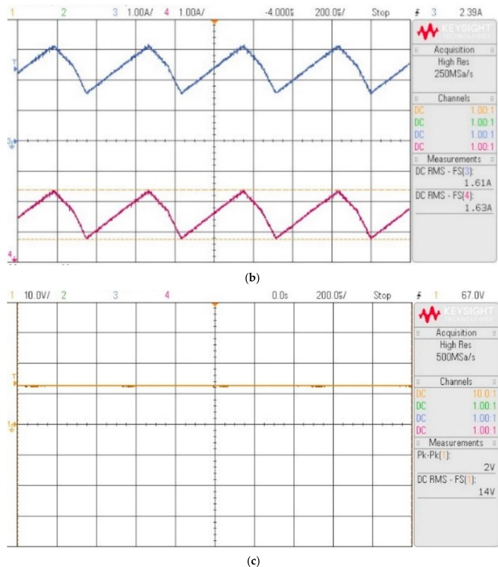
**Figure 10.** Output waveforms of step-down mode. (a) Output voltage and output current, (b) inductor voltage ( $I_{L1}$  and  $I_{L2}$ ), and (c) capacitor voltage ( $V_{C1}$ ).
