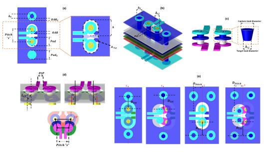
**Figure 3.** Sketch of the geometrical parameters (**a**) Planar view and parameters for the differential pair and the stitching couple (**b**) Nomenclature for the diameters and PtP distances (**c**) Diameters for the capture land and target land of the VIA (**d**) Front view and parameters taking into account the slant (**e**) Stitching VIA parameters.
