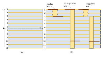
**Figure 2.** Reference structures: (a) An N = 12 layer stack-up; (b) different VIA structures.
