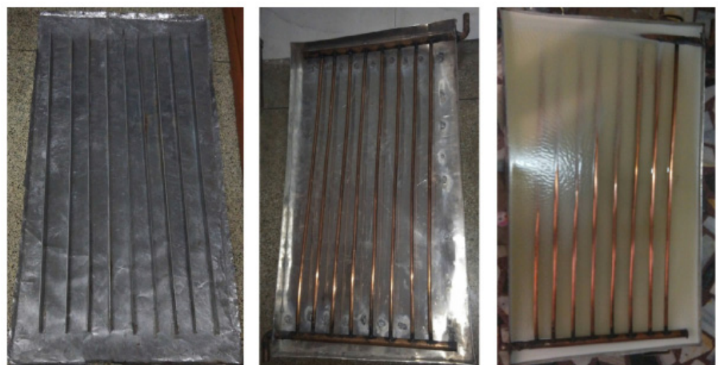
Figure 10. Diagram of three types of absorber plate used by Zhou et al. [36].
