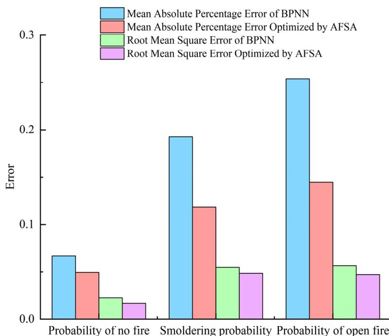
**Figure 6.** Error of BPNN and AFSA-BPNN algorithms in predicting fire probability.
