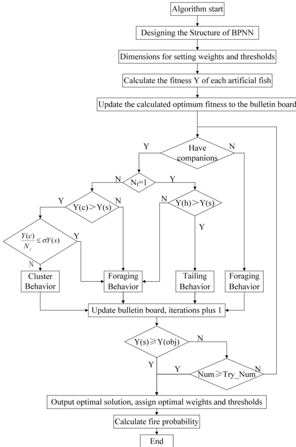
Figure 3. AFSA for optimizing flow chart of BPNN.
