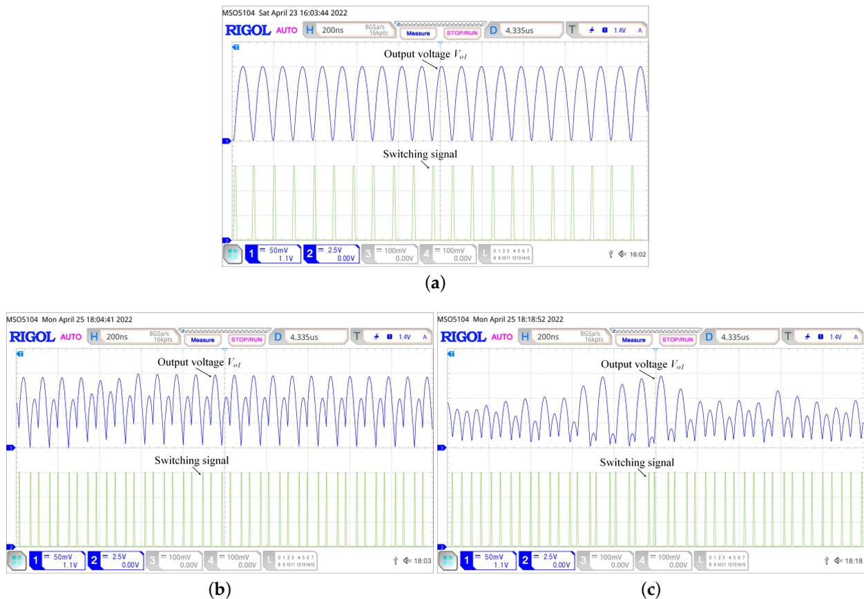
**Figure 10.** Experimental waveforms of the system with varying: (a)  $P_{CPL} = 6$  W. (b)  $P_{CPL} = 24$  W. (c)  $P_{CPL} = 33.1$  W.
