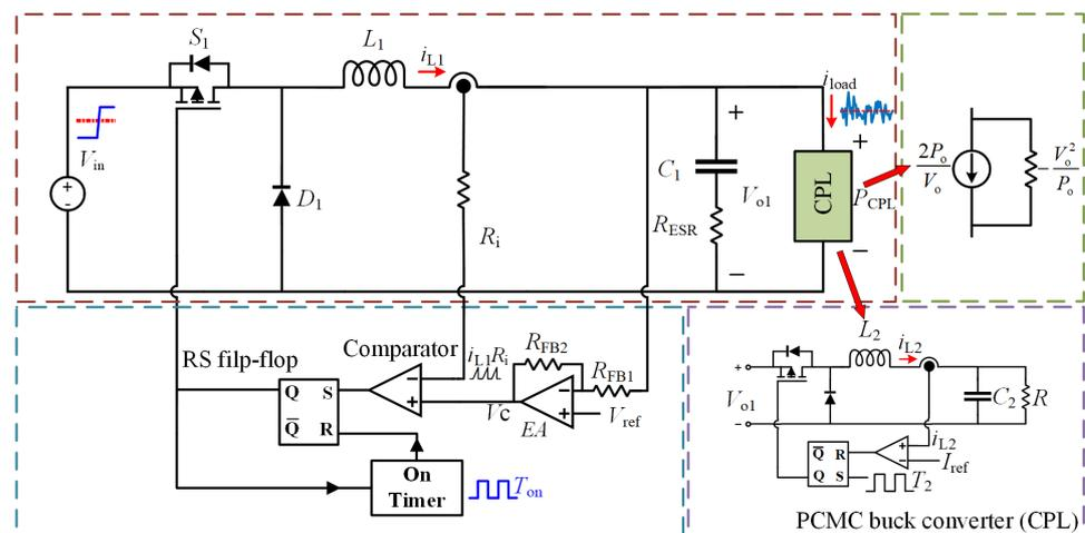
Figure 2. The prototype dual-stage cascaded dc system.
