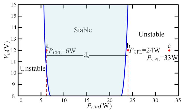
**Figure 4.** Stability boundary of the system as  $V_{in}$  varies from 8 to 16 V and  $P_{CPL}$  varies from 0 W to 35 W.
