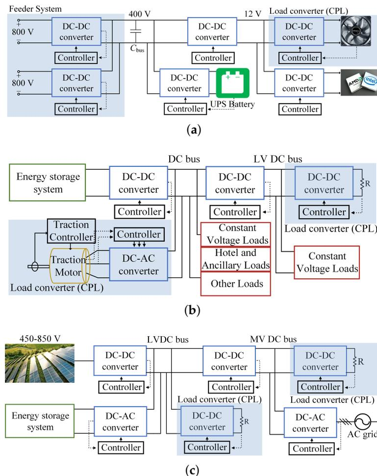
**Figure 1.** Some typical dual-stage cascaded dc systems [7,8]: (a) Data center dc power supply system. (b) Plug-in hybrid vehicle power supply system. (c) PV-storage integrated grid connected power supply system [7,8].
