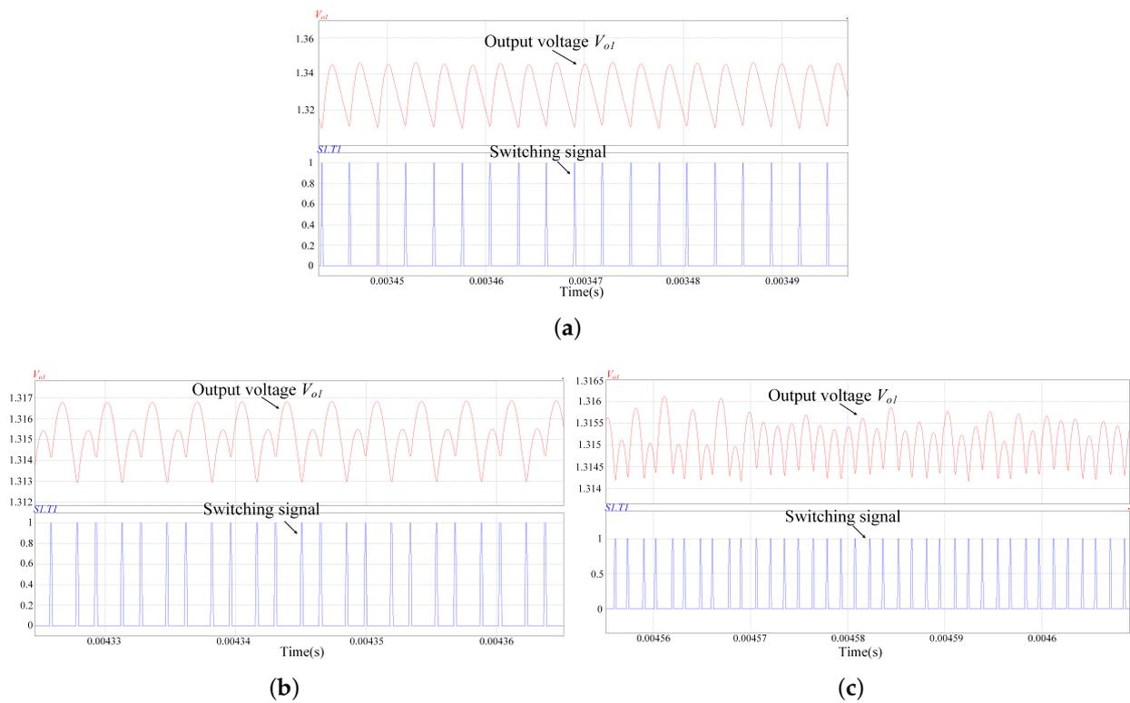
**Figure 8.** Simulation waveforms of the system with varying: (a)  $P_{CPL} = 6$  W. (b)  $P_{CPL} = 24$  W. (c)  $P_{CPL} = 33.1$  W.
