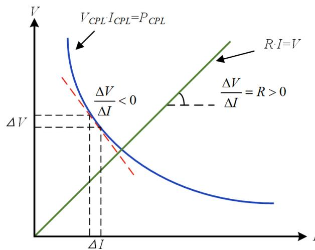
Figure 3. V-I characteristics of CPL and conventional resistive load [7].
