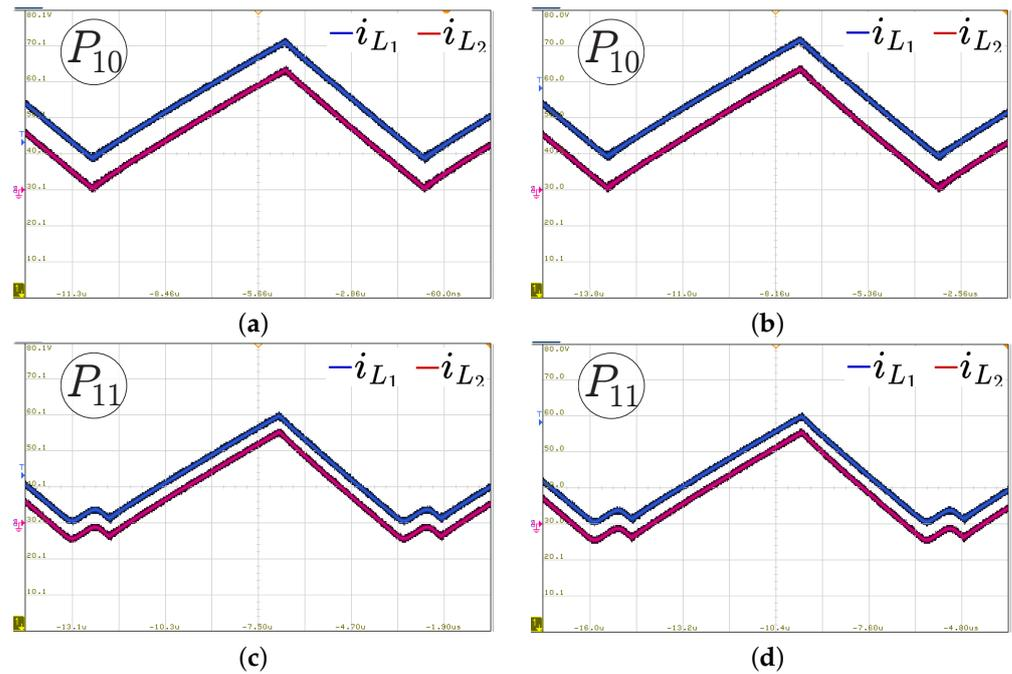
Figure 17. Inductor current waveforms in a closed-loop control with a voltage conversion ratio of 1.4: (a) SEPIC in point  $P_{10}$ , (b) Ćuk in point  $P_{10}$ , (c) SEPIC in point  $P_{11}$ , and (d) Ćuk in point  $P_{11}$ , (400 mA/div, DC coupling, and a time base of 1.4  $\mu$ s).
