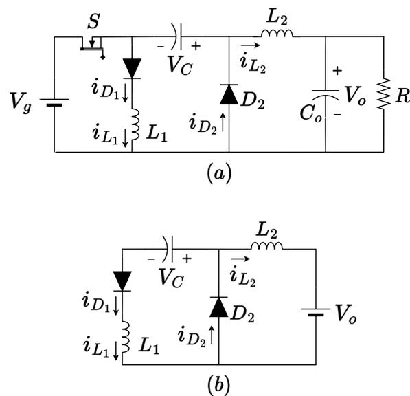
Figure 7. (a) Zeta-modified converter a with diode at the input port  $L_2$ , (b) equivalent circuit when the transistor is OFF.
