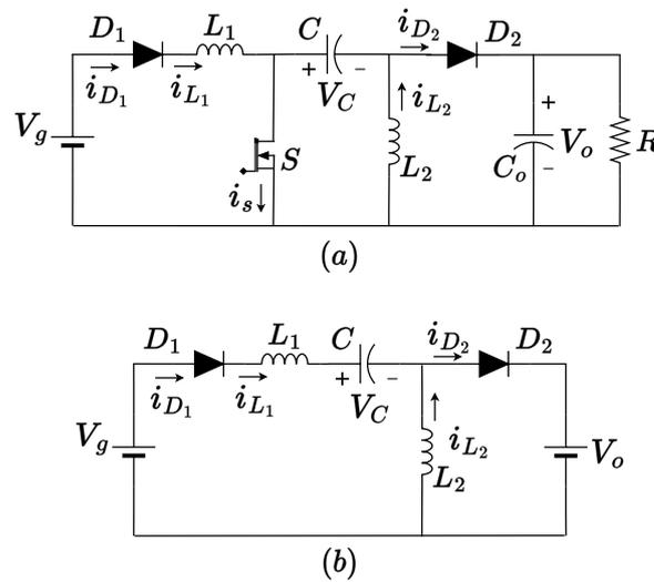
**Figure 2.** (a) SEPIC converter modified with an additional diode at the input port, (b) equivalent circuit when the transistor is OFF.
