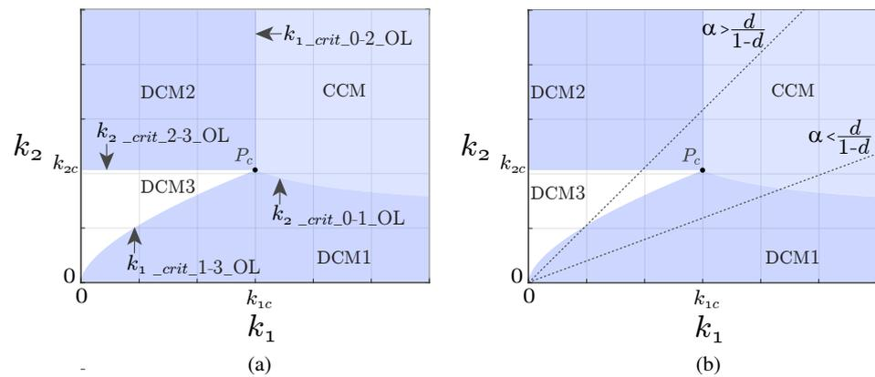
Figure 4. (a) Map of conduction regions in an open loop, (b) possible trajectories.
