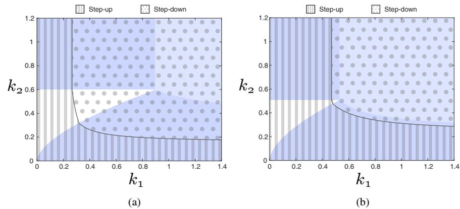
Figure 10. Step-down and step-up borders with constant duty cycles: (a)  $d = 0.4$ , (b)  $d = 0.49$ .
