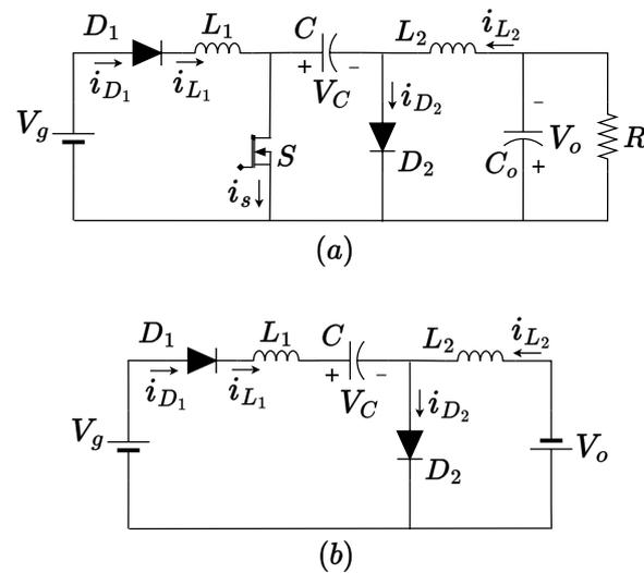
**Figure 6.** (a) Ćuk modified converter with a diode at the input port, (b) equivalent circuit when the transistor is OFF.
