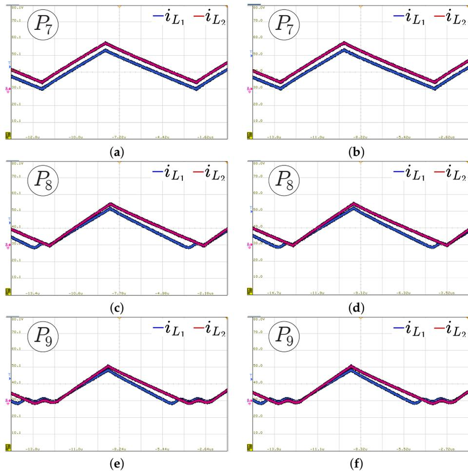
**Figure 16.** Inductor current waveforms in the closed-loop control with a voltage conversion ratio of 0.7: (a) SEPIC in point  $P_7$ , (b) Ćuk in point  $P_7$ , (c) SEPIC in point  $P_8$ , (d) Ćuk in point  $P_8$ , (e) SEPIC in point  $P_9$ , and (f) Ćuk in point  $P_9$ , (400 mA/div, DC coupling, and a time base of 1.4  $\mu$ s).
