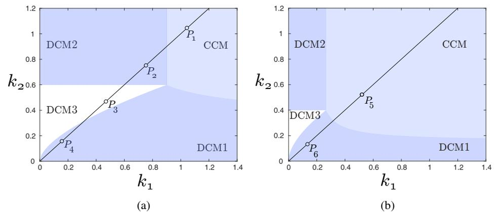
**Figure 12.** Map of the conduction regions in an open loop for either SEPIC or Ćuk converters: (a)  $d = 0.4$  and (b)  $d = 0.6$ . The points corresponding to the experimental results are highlighted.
