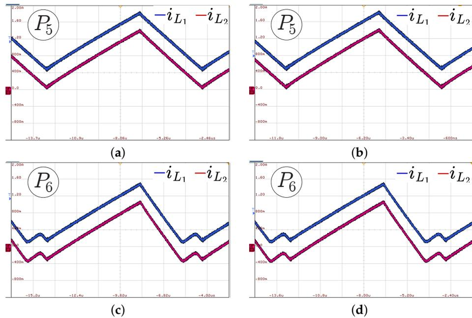
**Figure 15.** Inductor current waveforms in the open-loop control with a duty cycle of 0.6: (a) SEPIC in point  $P_5$ , (b) Ćuk in point  $P_5$ , (c) SEPIC in point  $P_6$ , and (d) Ćuk in point  $P_6$ , (400 mA/div, DC coupling, and a time base of 1.4  $\mu$ s).
