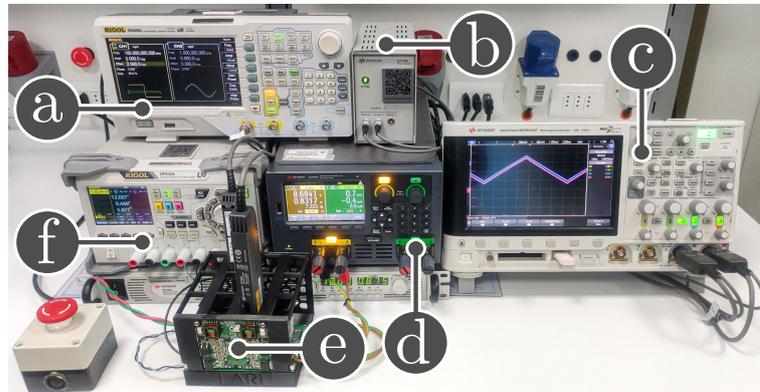
**Figure 11.** Experimental setup for testing in SEPIC and Ćuk converters: (a) arbitrary waveform generator to program the duty cycles, (b) auxiliary power supply to current probes, (c) oscilloscope, (d) electronic load, (e) reconfigurable prototype, and (f) DC power source.
