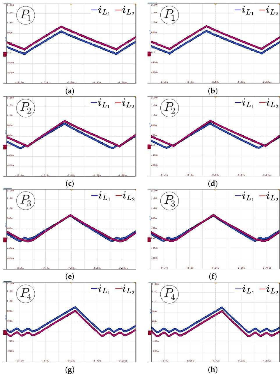
**Figure 14.** Inductor current waveforms in the open-loop control with a duty cycle of 0.4: (a) SEPIC in point  $P_1$ , (b) Ćuk in point  $P_1$ , (c) SEPIC in point  $P_2$ , (d) Ćuk in point  $P_2$ , (e) SEPIC in point  $P_3$ , (f) Ćuk in point  $P_3$ , (g) SEPIC in point  $P_4$ , and (h) Ćuk in point  $P_4$ , (400 mA/div, DC coupling, and a time base of 1.4  $\mu$ s).
