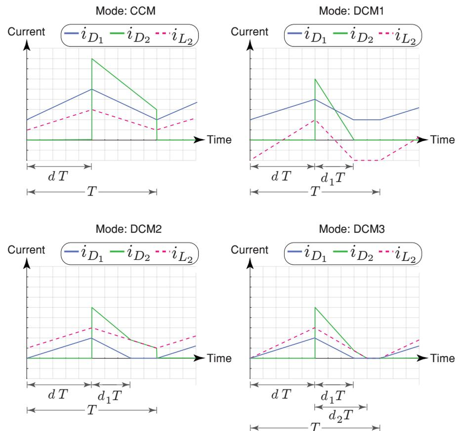
Figure 3. Current waveforms in each conduction mode.
