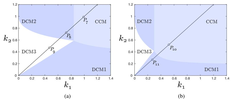
**Figure 13.** Map of conduction regions in closed loops for either SEPIC or Ćuk converters: (a)  $M = 0.7$  and (b)  $M = 1.4$ . The points corresponding to the experimental results are highlighted.
