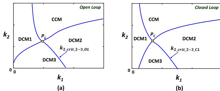
Figure 1. Example of the  $k$ -space for  $n = 2$ : (a) open loop, (b) closed loop.
