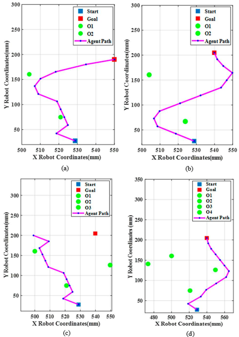
Figure 15. Path Traversed by the Robot using Double DQN (a) With Two Obstacles, (b) With Two Obstacles for Different Goal Positions, (c) With Three Obstacles, and (d) With Four Obstacles. The Yellow Colored Arrow Illustrates the Path taken by the Agent.
