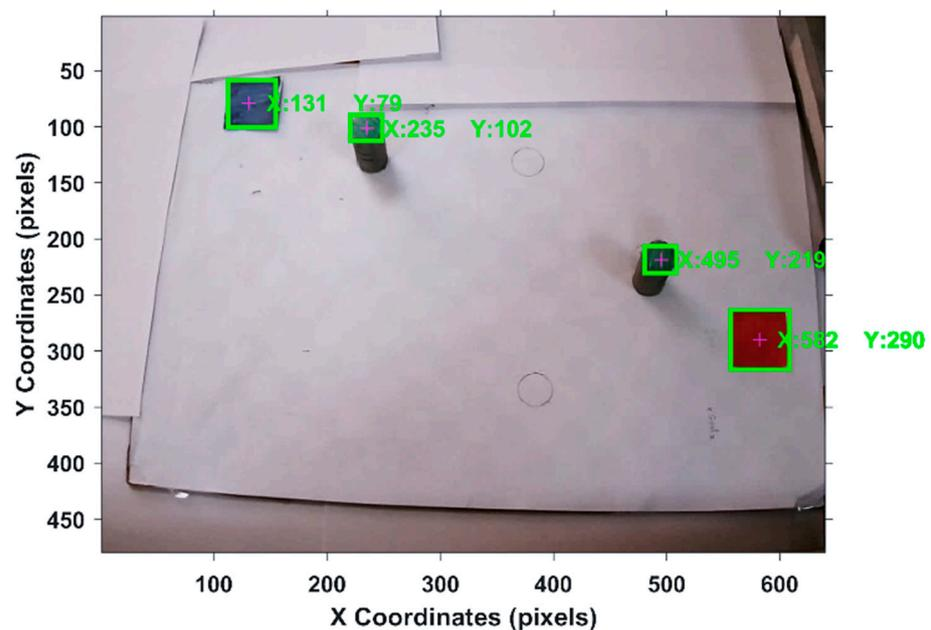
Figure 9. Live Camera Feed With Start, Goal, and Obstacle Positions for Online Vision-Based Path Planning.
