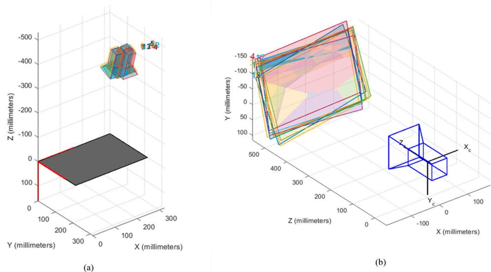
Figure 2. (a) Pattern Centric View of Eye-to-Hand Calibration (b) Camera Centric View of Eye-to-Hand Calibration.
