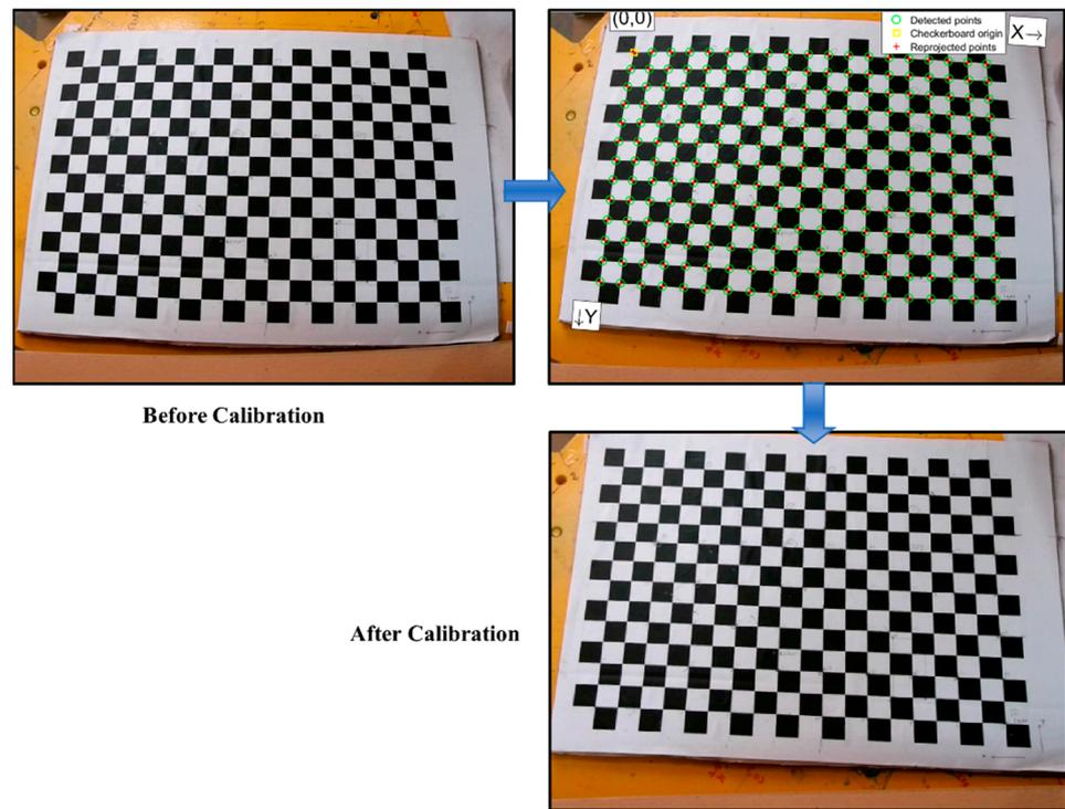
Figure 1. Calibration of Eye-to-Hand Camera Tilted at  $26^\circ$ .
