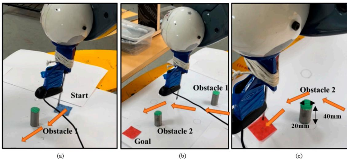
**Figure 16.** Real-time Path Traversed by the Robot with Two Obstacles using Double DQN (a) At Start Position (Blue), (b) At Middle Position, and (c) Goal Position (Red). The Yellow Colored Arrow Illustrates the Path taken by the Agent.
