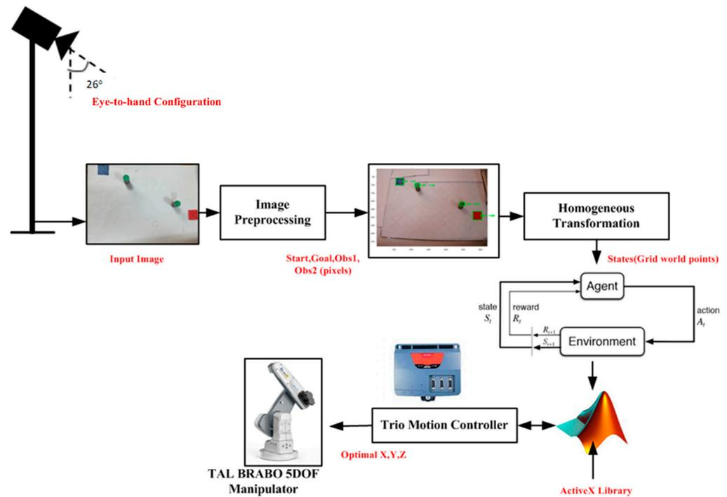
**Figure 4.** Process Flow of Vision-Based Obstacle Avoidance using Different Reinforcement Learning Algorithms.
