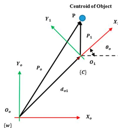
**Figure A2.** Transformation of Centroid Points P from Camera Frame to Grid World Coordinates.
