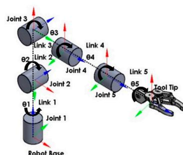
**Figure A1.** Kinematic Diagram of TAL BRABO Manipulator.
