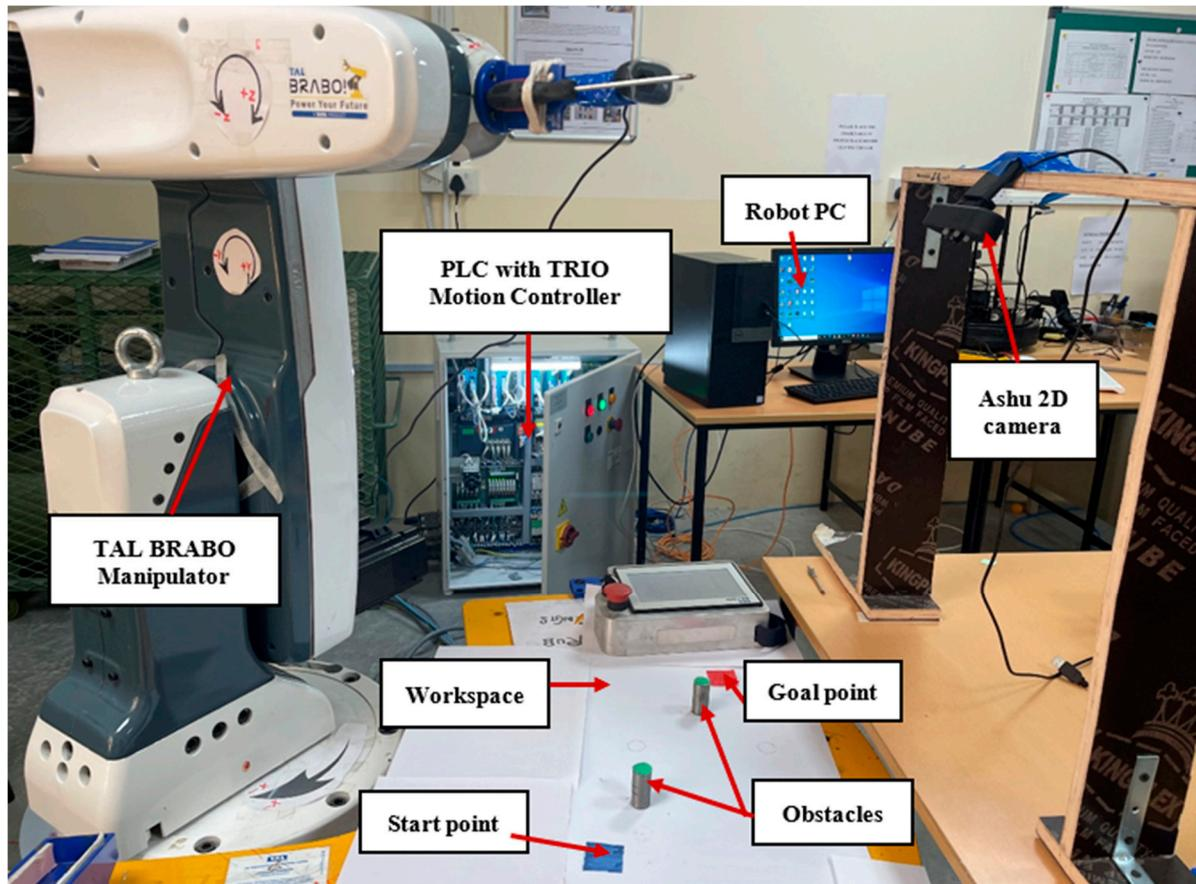
Figure 8. Experimental Setup for Vision Based Path Planning Using Reinforcement Learning.
