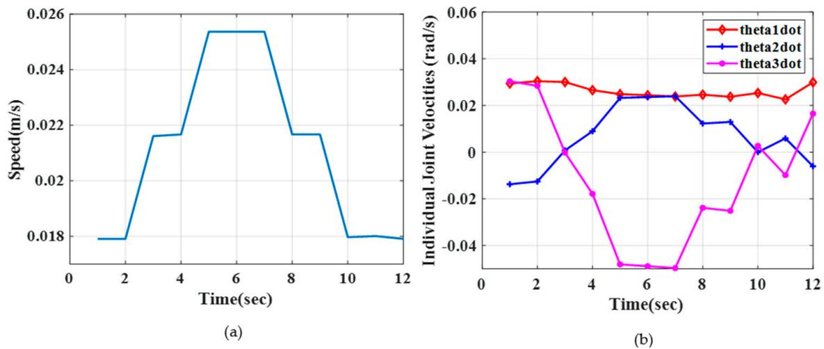
**Figure 17.** (a) Real-time Path Speed Profile of the Robot with Two Obstacles using Double DQN (b) Real-time Joint Velocities of the Robot with Two Obstacles using Double DQN.
