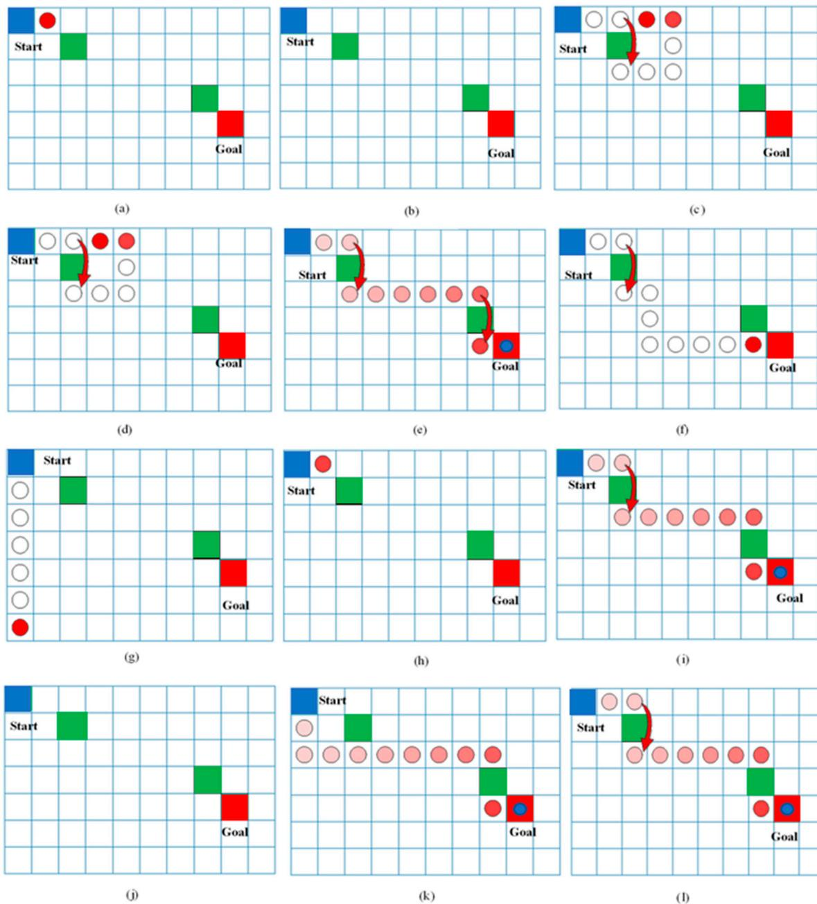
**Figure 13.** Path Traversed by the Agent with  $E = 5000$  and Varying Discount Rate (a–c) Q-Learning (d–f) SARSA (g–i) DQN (j–l) Double DQN. Also, in some cases like in Figure (b,j) and Figure (c,d), there was no change in path or the agent does not respond at all.
