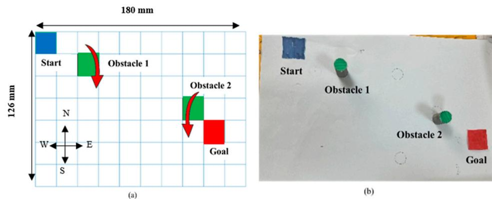
**Figure 5.** (a) Simulated Grid World Environment (b) Real-time Grid World Environment in Robot Workspace.
