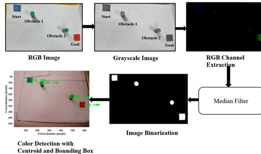
**Figure 3.** Process Flow of Color Detection using Image Processing Techniques.
