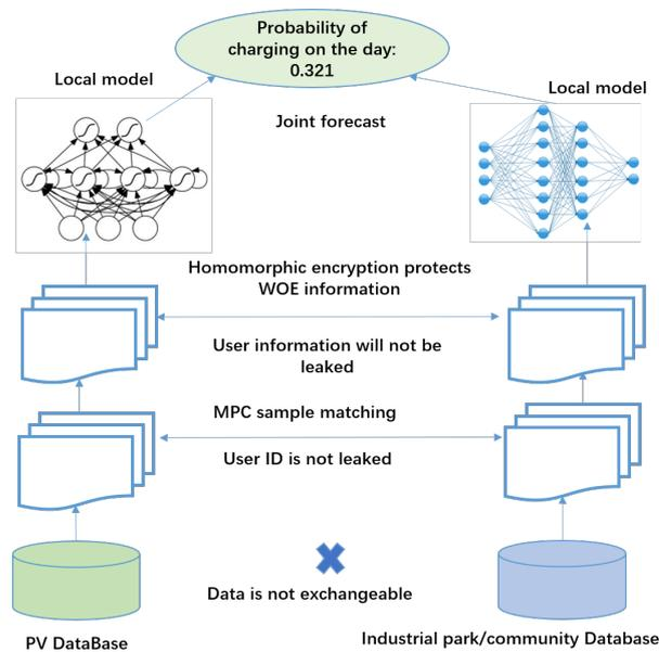
Figure 4. Calculating EV charging probabilities with federated learning.
