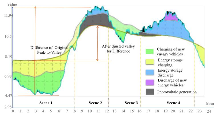
**Figure 9.** Scenario application of A charging station—expectation of an EV participating in DR and operation characteristics. (1) Pure load + energy storage + photovoltaic + new energy vehicles, participate in the scene application. (2) The interaction effect of EVs participating in the power grid: the original peak valley difference is 7.53 MW, and the adjusted peak valley difference is 2.98 MW, reducing the peak valley difference.
