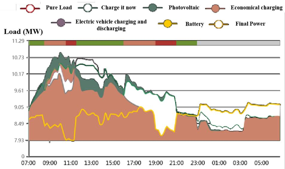
Figure 11. Photovoltaic, EVs, and energy storage coordinate peak-shaving and valley-filling.
