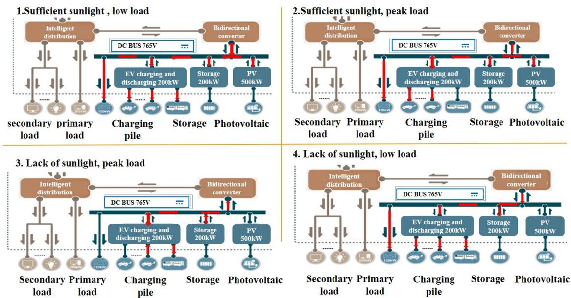
**Figure 7.** Typical operation mode of interaction and energy balance between new energy vehicles and distributed new energy.
