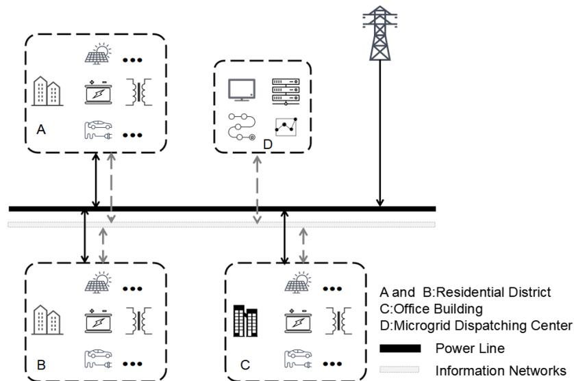
Figure 5. Application scenario diagram.
