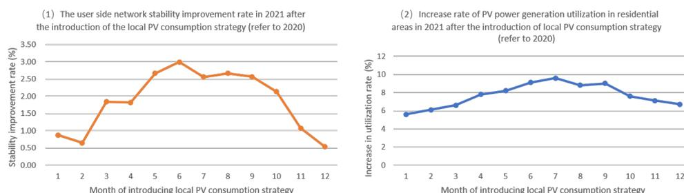
**Figure 13.** Introducing electric vehicle charging and energy storage to participate in the performance analysis and evaluation of the residential distributed photovoltaic power generation absorption strategy (absorption capacity, power supply stability).
