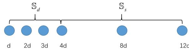
Figure 1. Nested array configuration with  $R = 6, M = 2, N = 4$ .
