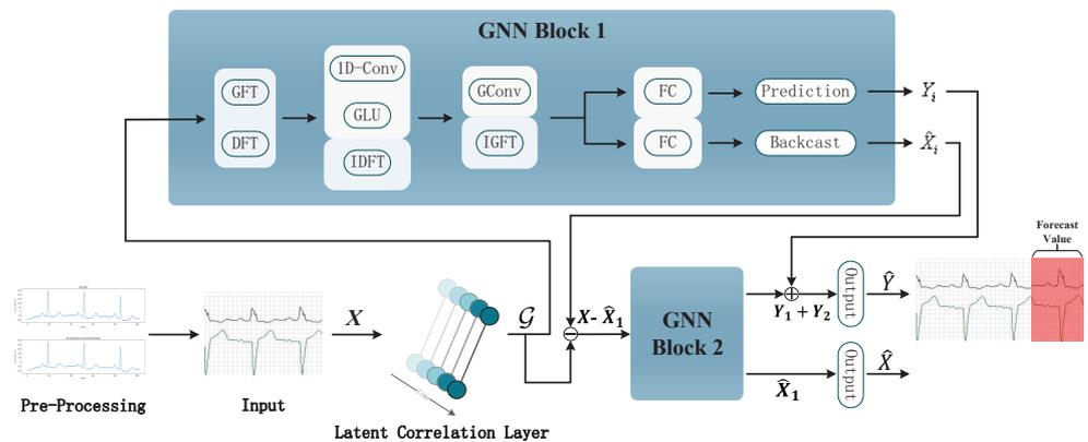
Figure 1. The overall architecture of Graph Neural Network.
