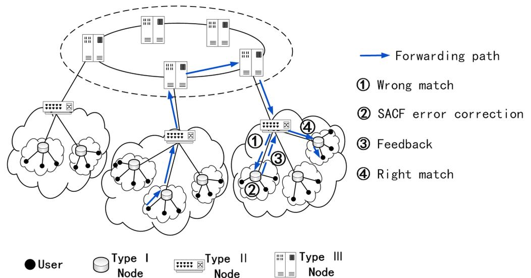
Figure 5. Error correction feedback mechanism.
