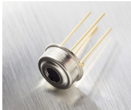
Figure 5. Melexis MLX90614: an infrared thermometer for non-contact temperature measurements [36].
